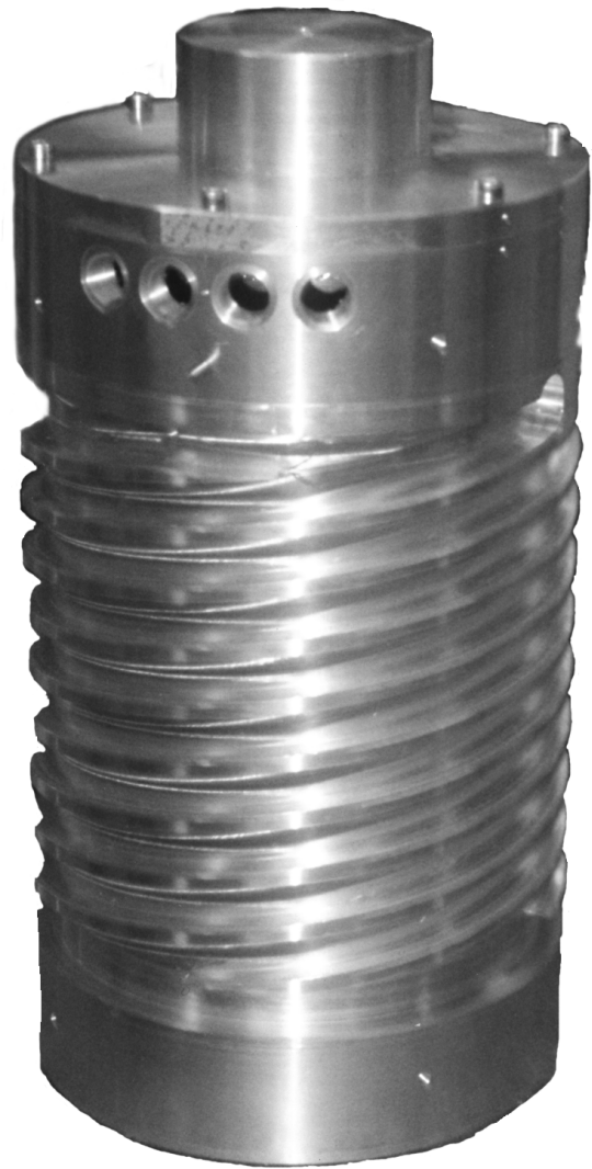
Figure 2: The stator frame during manufacturing
