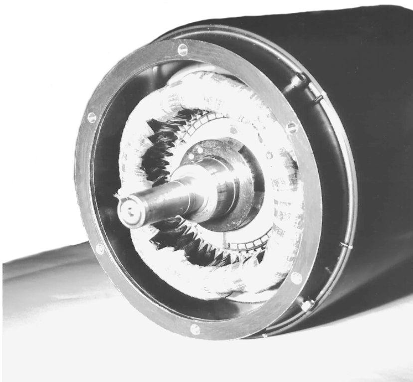
Figure 2: A view from the drive end of the experimental motor
