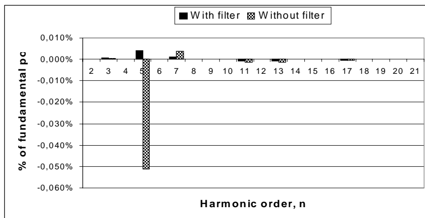
Figure 5.3.7. Harmonic active power on transformer secondary side.
