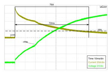
Figure 4.5: Example of a start up pulse approximated with one square.
