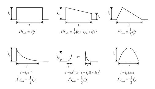
Figure 4.1: Different wave shapes used when approximately calculating the energy of a current pulse.
