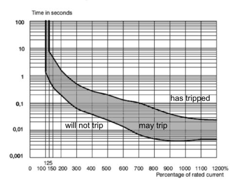
Figure 4.3: A time current curve
