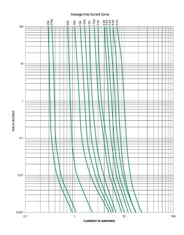
Figure 2.4: A time-current curves for melting fuses. Figure reproduced with the courtesy of Littlefuse Inc.
