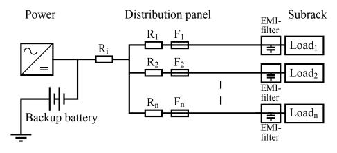
Figure 2.12: Two step high ohmic distribution
