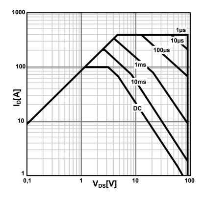
Figure 2.10: A typical safe operating area curve of a MOSFET
