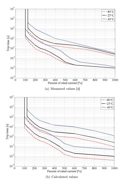
Figure 4.2: Comparison of a calculated and measured value of influence of ambient temperature on trip time for a magnetic hydraulic circuit breaker.
