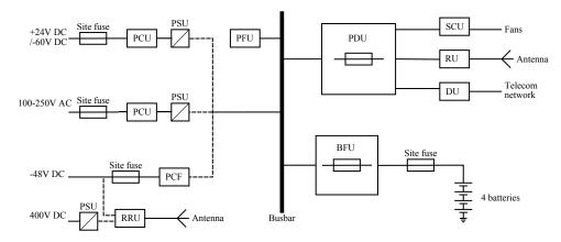
Figure 2.11: Power system hardware units and interfaces of a radio base station.
