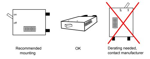
Figure 4.8: Recommended mounting of a magnetic hydraulic circuit breaker.
