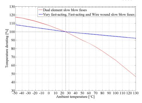
Figure 2.2: Temperature derating of melting fuses.
