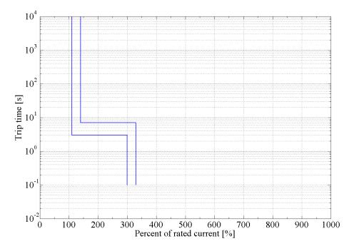
Figure 4.10: Trip characteristics of an electronic fuse.
