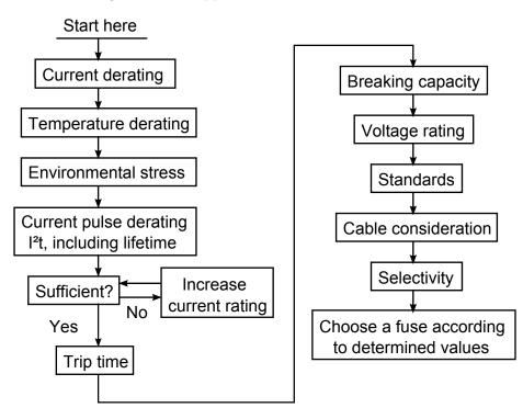
Figure 4.11: Flow chart when choosing a melting fuse.
