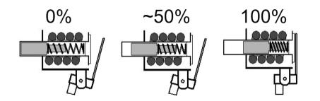
Figure 4.4: Core positions in the coil
