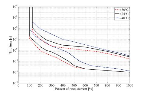
Figure 2.7: An example of the influence of ambient temperature for a magnetic hydraulic circuit breaker.
