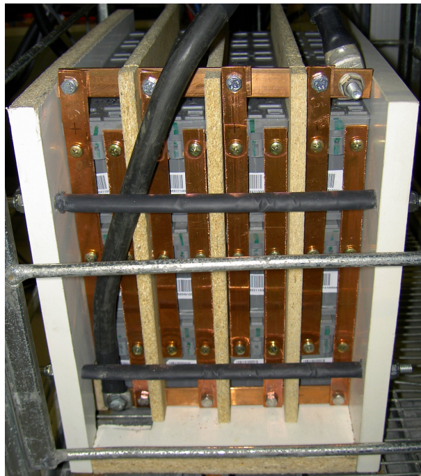
Figure 19: Photo of the support battery used in measurements with single supercapacitors.
