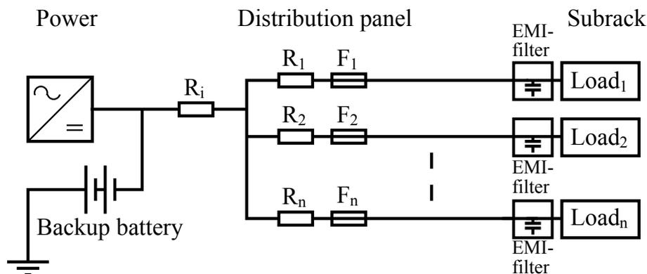
Figure 2.12: Two step high ohmic distribution
