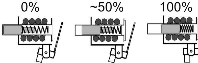
Figure 4.4: Core positions in the coil
