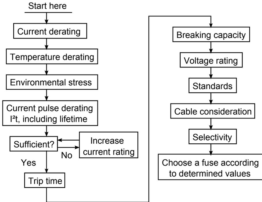
Figure 4.11: Flow chart when choosing a melting fuse.
