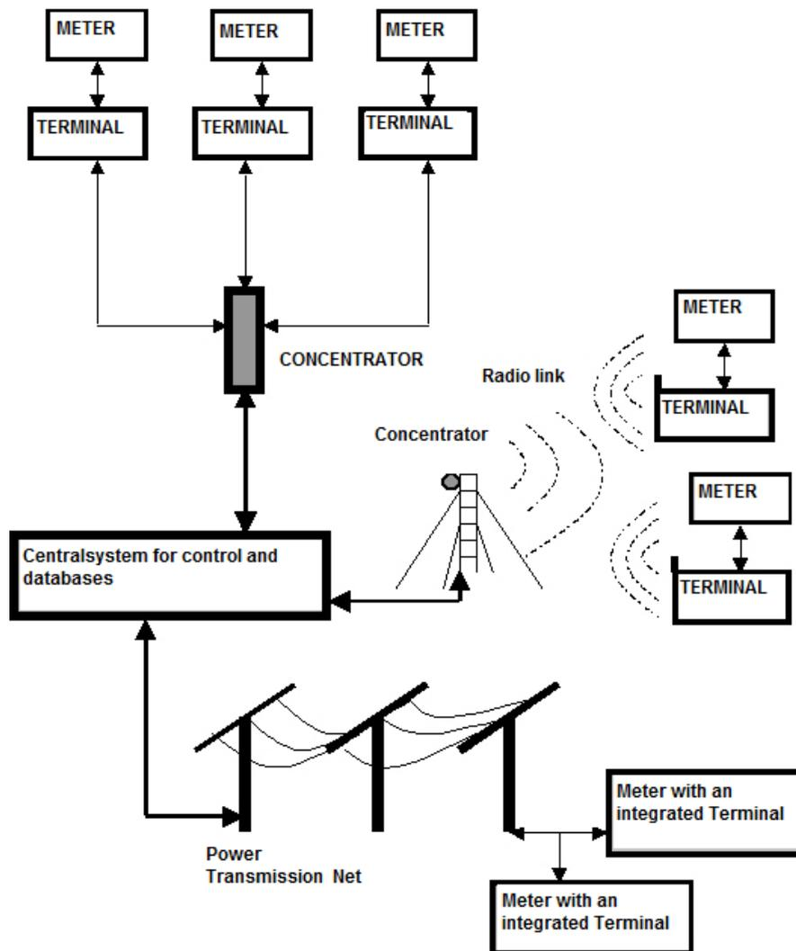
**Figure 3 Schematic overview of a smart metering system.**
