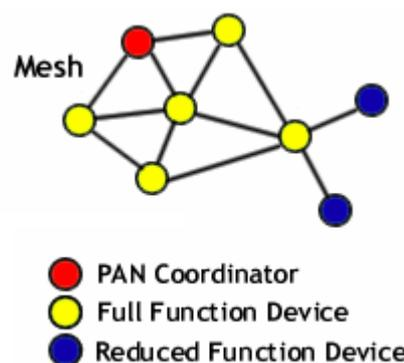
**Figure 6 Structure of a mesh network.**
