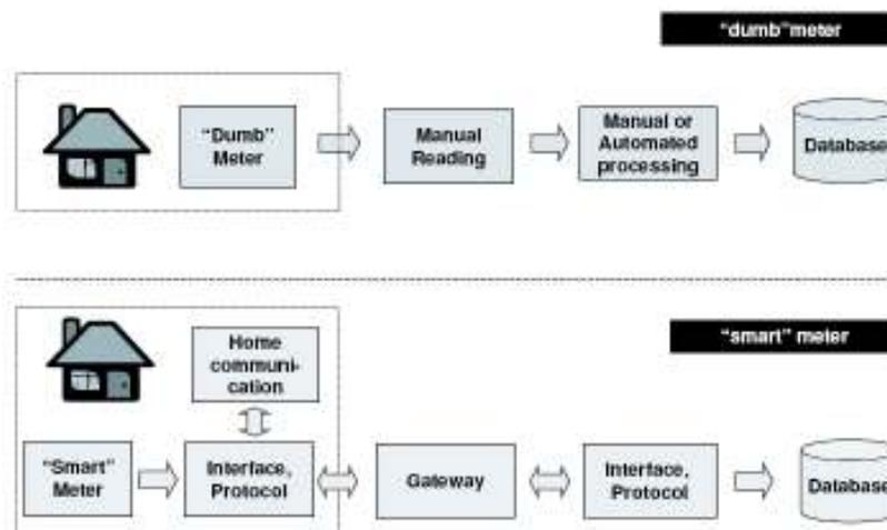
Figure 2 Comparison between an old "dumb" meter and a new "smart" meter [12].
