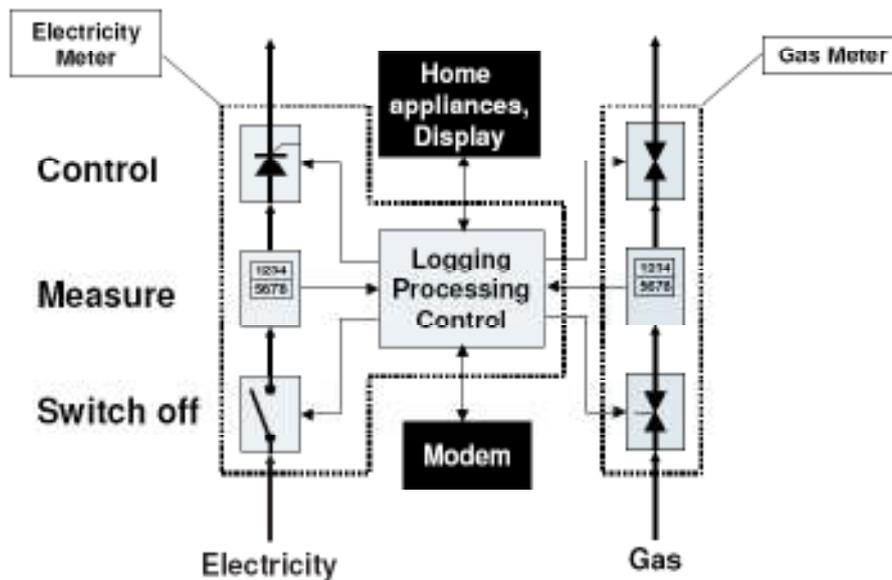
Figure 1 Overview of a smart meter configuration [12].
