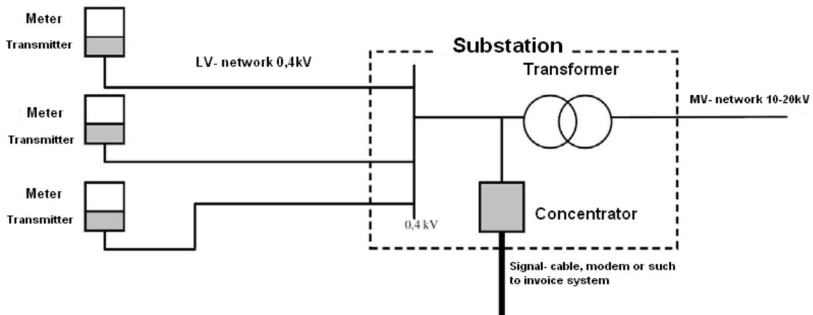
Figure 5 Low voltage PLC communication system.
