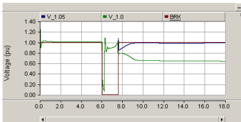
Figure 28 Voltage recovery with switched shunt capacitor
