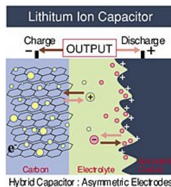
Figure 2.20: Structure of a Li-ion capacitor, [22]
