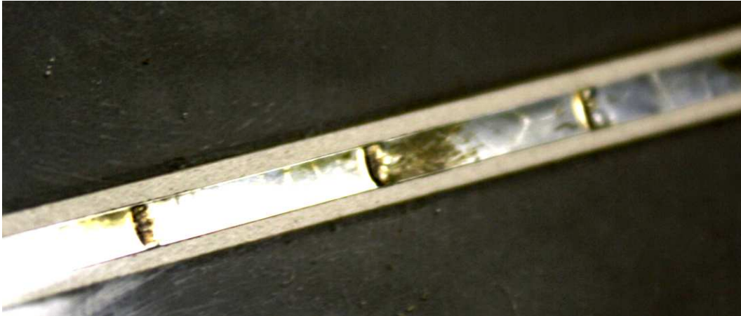
Figure 30. Corroded back side bus bar in the H3-A samples at 72 hours, this occurred at 96 hours for the H2 samples.
