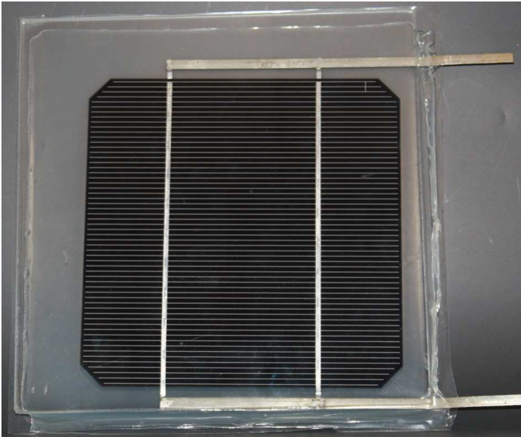
Figure 43. The back sheet foil slipped on the DH-B4.
