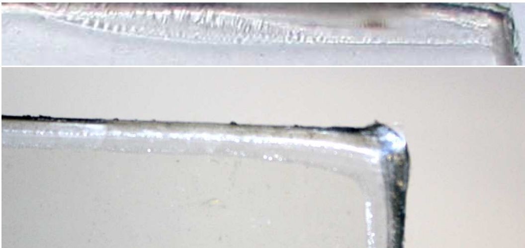
Figure 31. HAST 24 hours: A samples show some de-lamination at the edges similar to DH.
