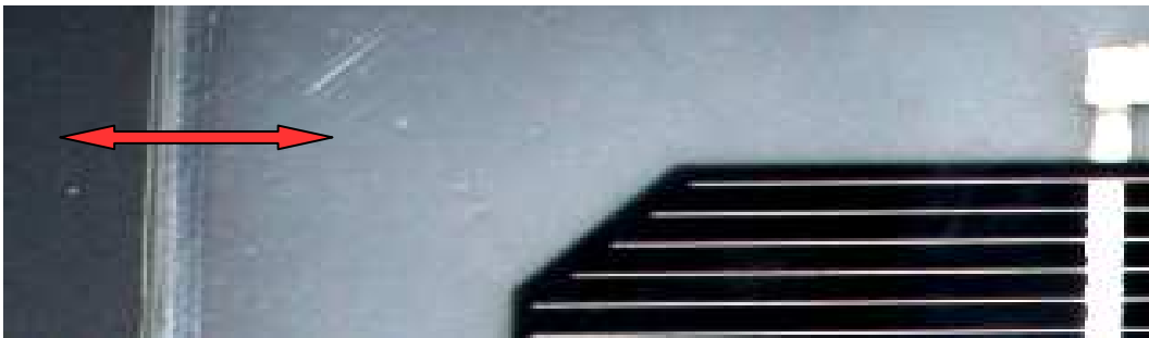
Figure 11. The sample A show a white haze after 500 hours, appearing after being all transparent at the beginning.
