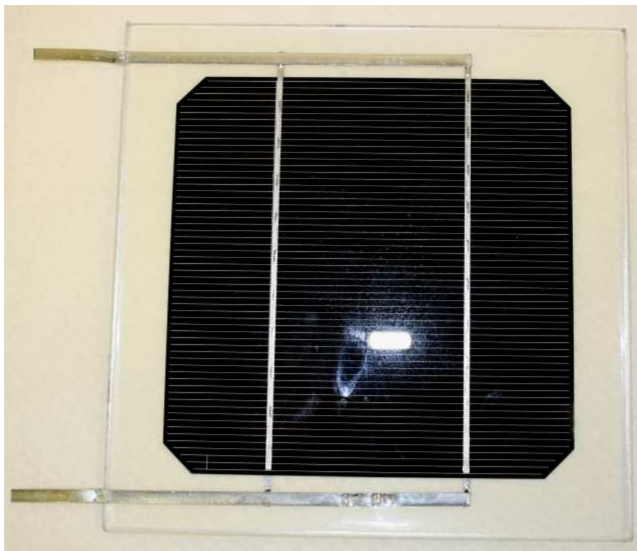
Figure 10. The typical module design for all samples.
