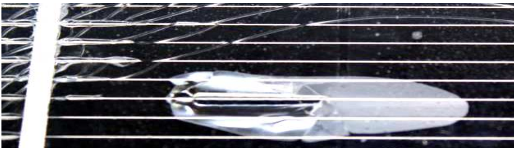
Figure 66. The C samples now de-laminate at the front side as well and not only at the bus bar.
