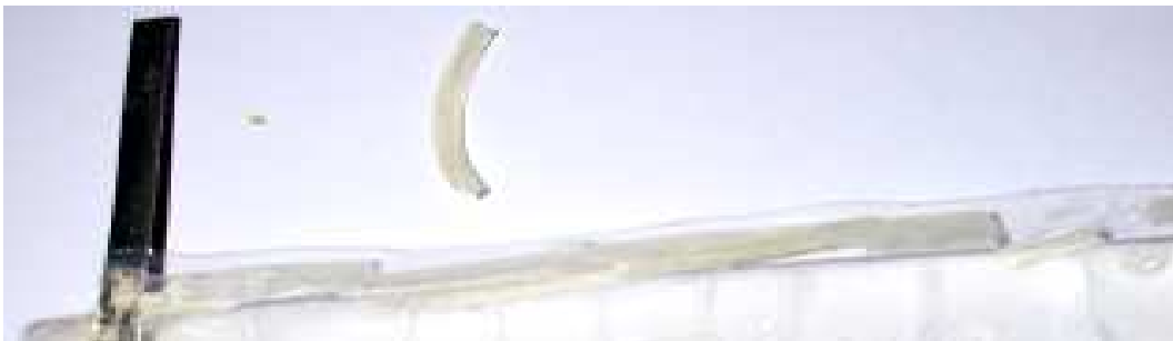
Figure 68. The thermoplastic falling out of the C samples.
