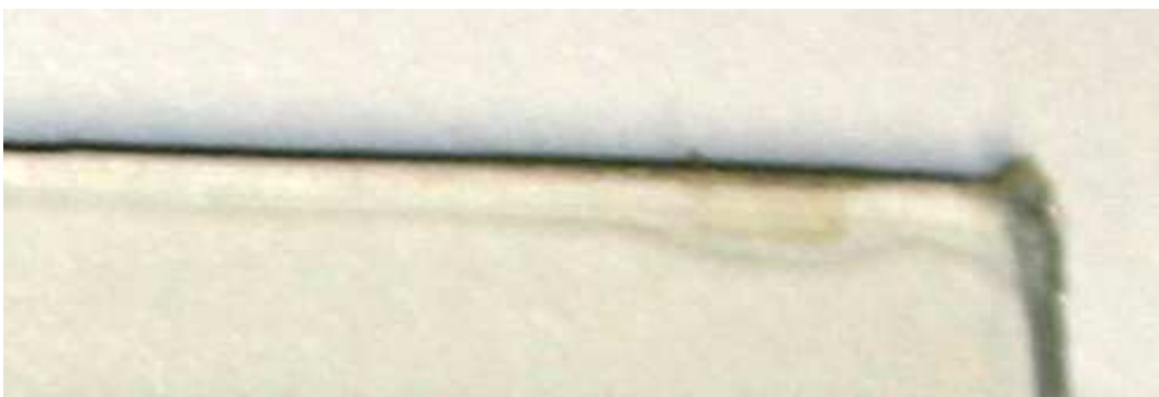
Figure 32. The same view of the A module at 48 hours. Now the embedding have a light browning but the bubbles does not seem to expand. The de-lamination at the edge is also seen.
