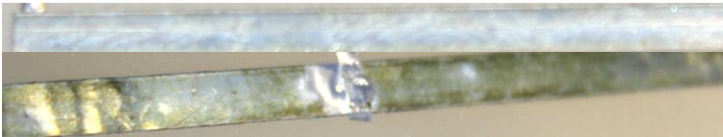
Figure 52. Clear front side of the leads but corrosion on the back side of the H2 leads after 72 hours HAST.
