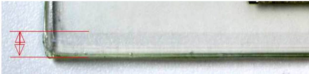
Figure 19. At the 2000 hours stage the sample A de-lamination at the edges is clear.
