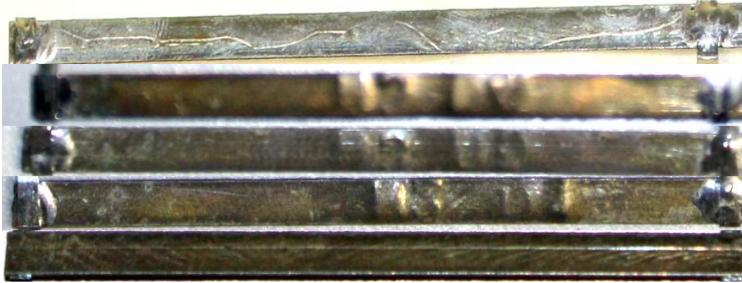
Figure 97. The corrosion development over 12, 24, 48, 72 and 96 hours in HAST
