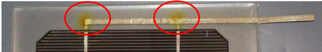
Figure 62. A typical view of the yellow spots on the C samples.
