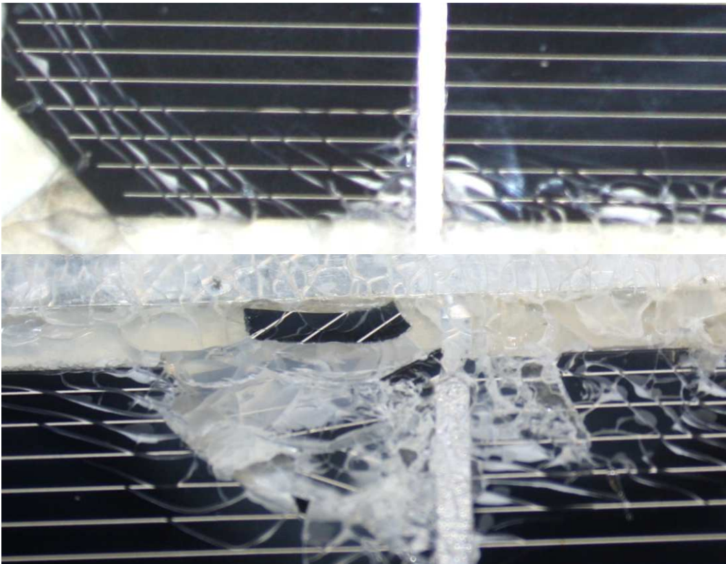
Figure 78. This is from the melted H3 samples after 48 hours. The front side start to de-laminate as well and some of the cells brake and flow out with the embedding material.
