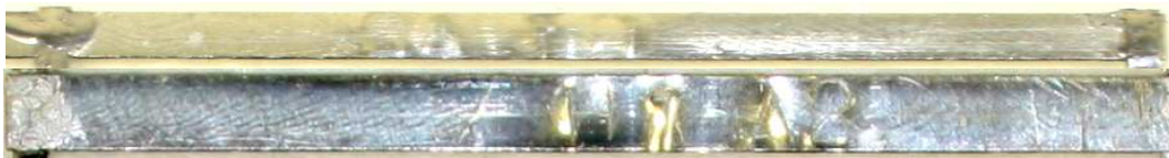
Figure 26. No corrosion after 12 hours.
