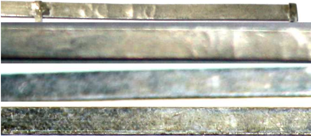
Figure 89. Corrosion after 500, 1000, 1500 and 2000 hours of DH, DH-D5.
