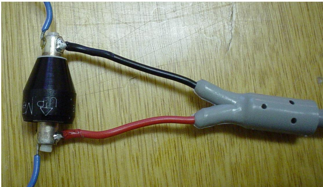
Figure 6.10 Soldered slip ring
