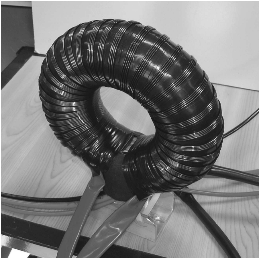
Fig. 7.8 The finished down scaled 5.6 kW transformer.
