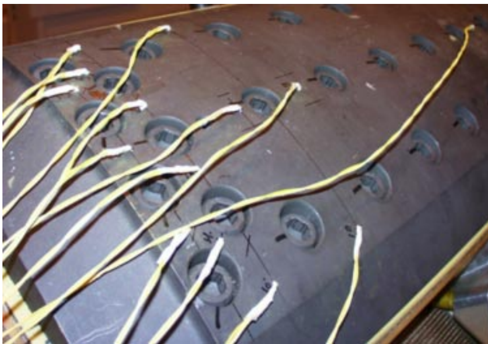
Figure 5.43 Some thermocouples on the rotor surface.
