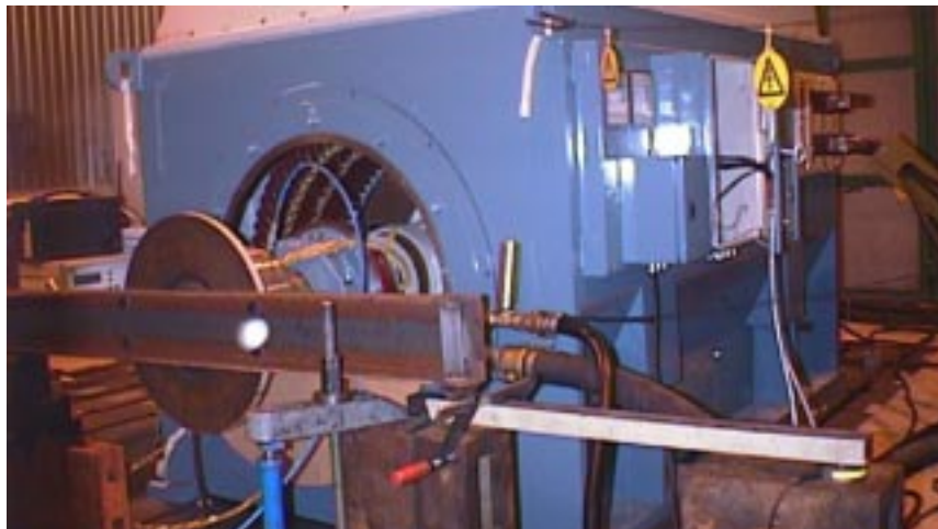
Figure 5.39 Torque lever and force sensor.
