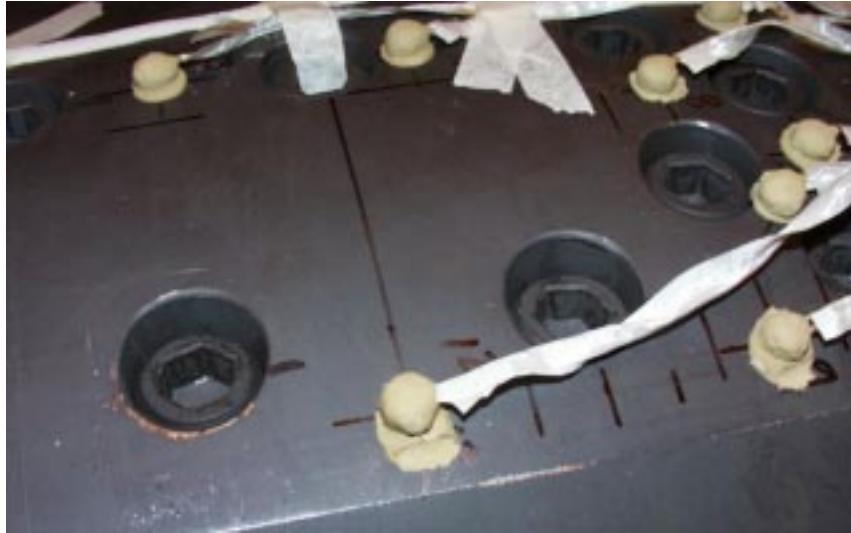
Figure 5.40 Some search coils glued to the rotor surface.
