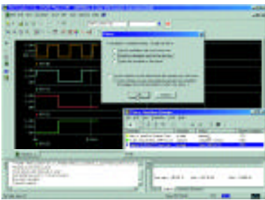
Pause a long simulation to run a shorter one. The Simulation Manager shows the current status of the simulations being performed.
