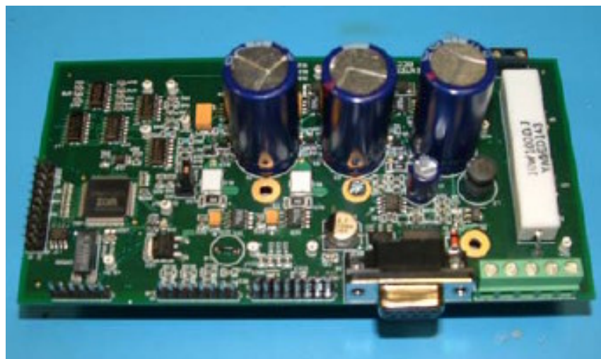
Figure 4.10 –physical view of sensor less PMSM driver, courtesy of IR
