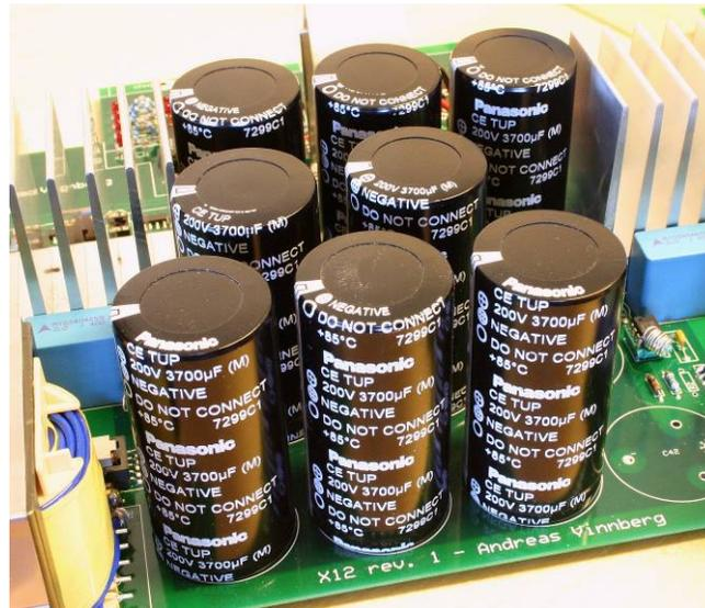
**Figure 26: Close up of primary capacitors**
