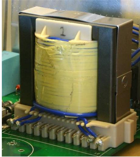
**Figure 27: Close-up of main transformer**
