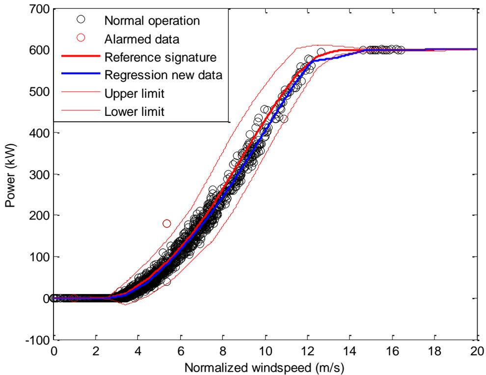
**Figure 5.11 Method of bins for parameterization and method of bins for alarm generation with a threshold set to  $2.5\sigma$ . The bin width is 1 m/s for both the reference signature and for the regression of new data up to 16 m/s. The width is thereafter enlarged for the new data. The data displayed is measured in the SSW direction, May 2010 - October 2010.**
