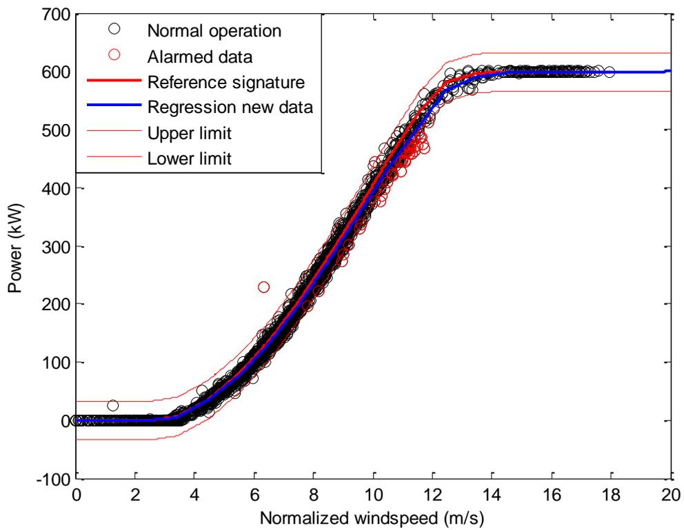
**Figure 6.2 Method of bins for parameterization and constant limit concept for alarms of data measured in direction W. An alarm factor of 3 is used, resulting in 47 alarms**
