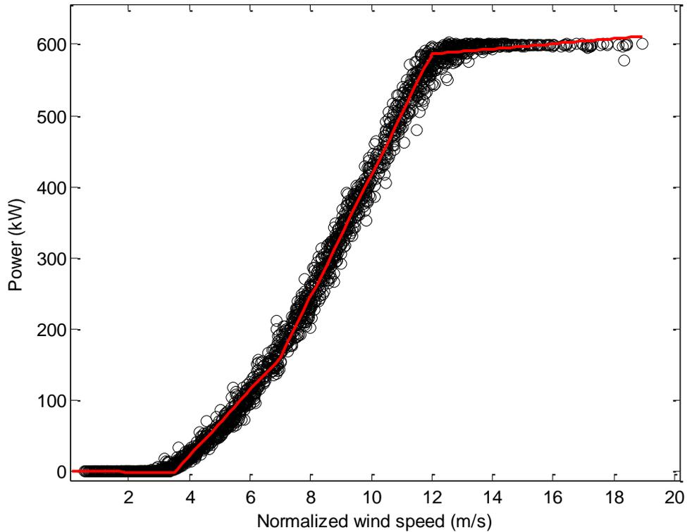
**Figure 5.2** Four-lines piecewise linear regression of data obtained from Boel in southerly (S) winds measured between 2008-07-01 and 2009-03-15. Knots are set at 3.5, 7 and 12 m/s.
