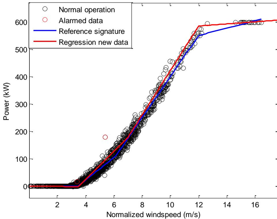
**Figure 5.10 Piecewise linear regression (4 lines) with piecewise limits concept for alarm initiating with an alarm threshold of  $5\delta$ . The data displayed is measured in the SSW direction, May 2010 - October 2010.**
