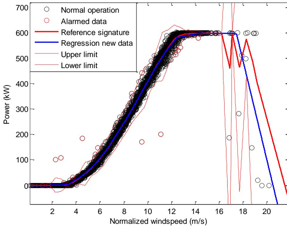
**Figure 7.6 Method of bins applied to data which has not been filtered. Method of bins is also used for alarm initiation. Data is measured at Boel in WSW direction.**
