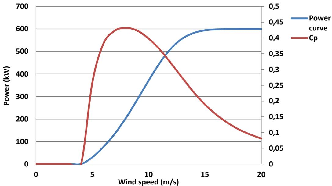
Figure 2.1 Power curve (blue line) and the power coefficient (red line) for Vestas V44-600 kW
