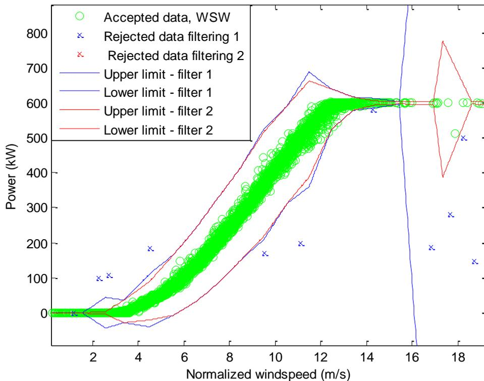
**Figure 5.1 Accepted and rejected data after the iterative filtering process for data measured in SSW direction at Boel.**
