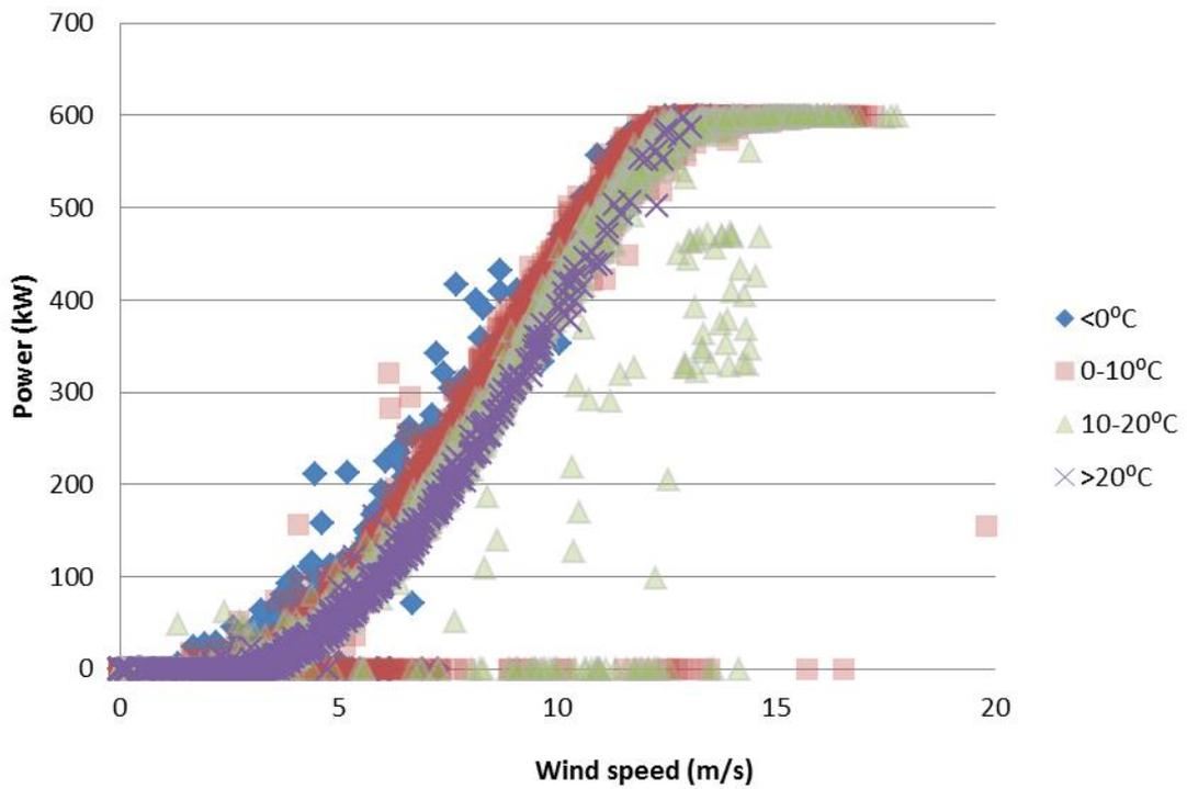
Figure 4.6 Power output from the wind turbine Boel for different temperature intervals.
