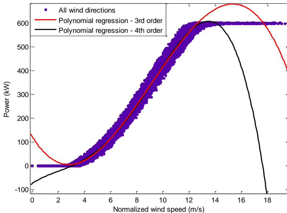
Figure 7.3 Parameterization of data, independently of wind direction.
