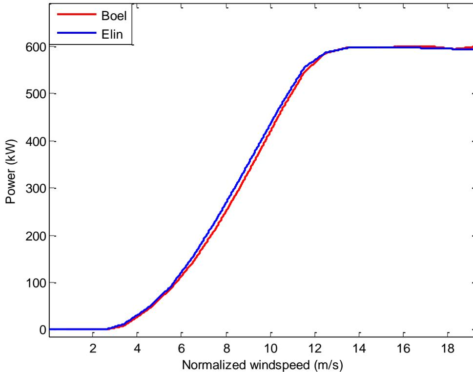
**Figure 7.4 Comparison of the signature of Boel and the signature of Elin based on data measured during the same period. The method of bins (1 m/s) was used to parameterize data measured in southerly (S) winds.**
