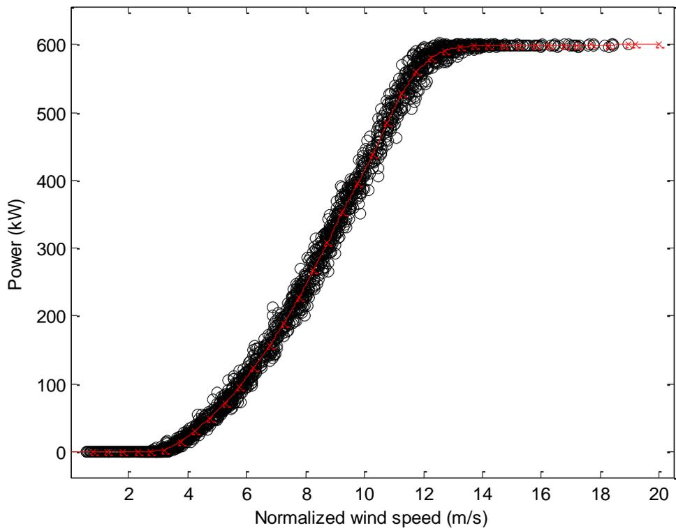
**Figure 5.7** Parameterization of data for Boel, using the method of bins with bins of 0.5 m/s each. Data is measured in southerly (S) winds from July 2008 until March 2009.
