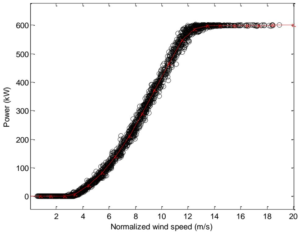
**Figure 5.6** Parameterization of data for Boel, using the method of bins with bins of 1 m/s each. Data is measured in southerly (S) winds from July 2008 until March 2009.
