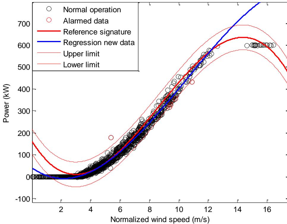
**Figure 5.9 Polynomial (3rd order) regression with constant limit concept for alarm initiating. The data displayed is measured in the SSW direction, May 2010 - October 2010. Data points outside of the upper and lower limit are considered as alarm.**
