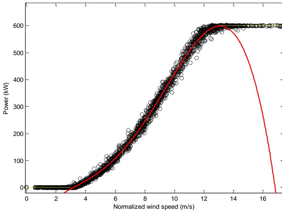
**Figure 5.5 Fourth order polynomial used for regression of wind power data measured at Boel between July 2008 and March 2009.**
