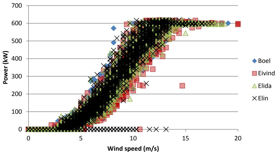
Figure 4.2 Power generated plotted against the wind speed measured at respectively turbine.
