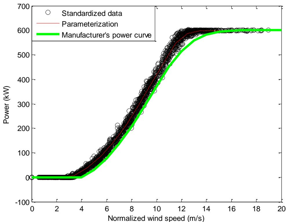
**Figure 7.5** Parameterized data from Boel compared to the power curve supplied by the manufacturer.
