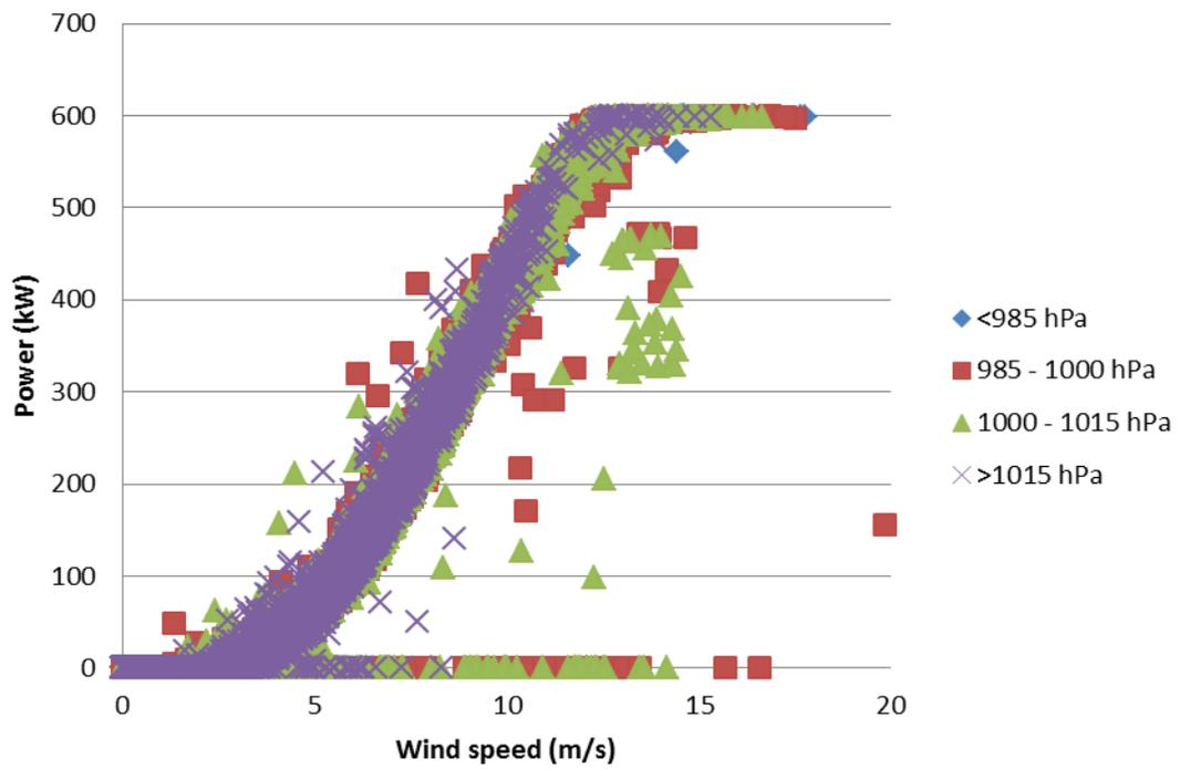
Figure 4.7 Power output for different pressure intervals.
