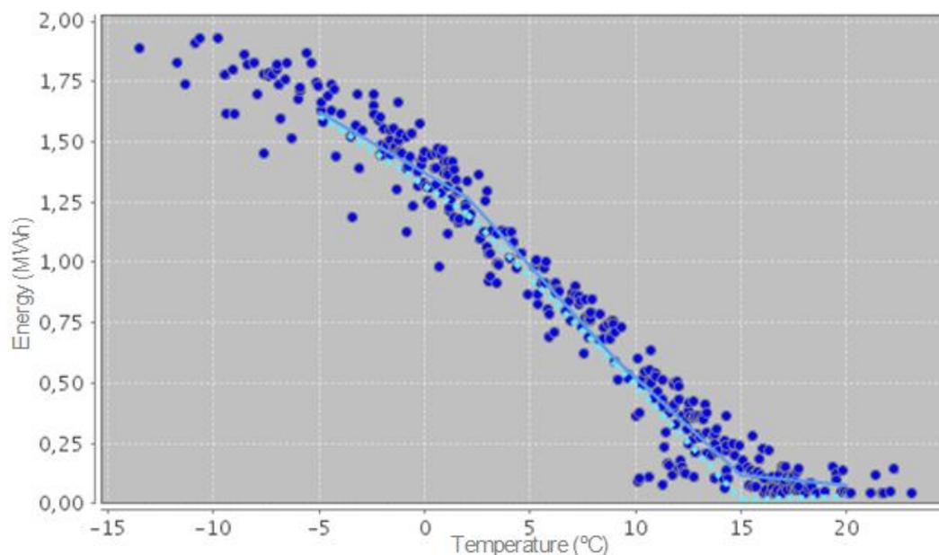
**Figure 3.1** Graph of supplied energy at different temperatures for a certain building obtained with Kasper. Dark blue dots are measured values from the last year. The dark blue line is the regression line resulting from the data points, the line of light blue dots is the reference line obtained from historic data.
