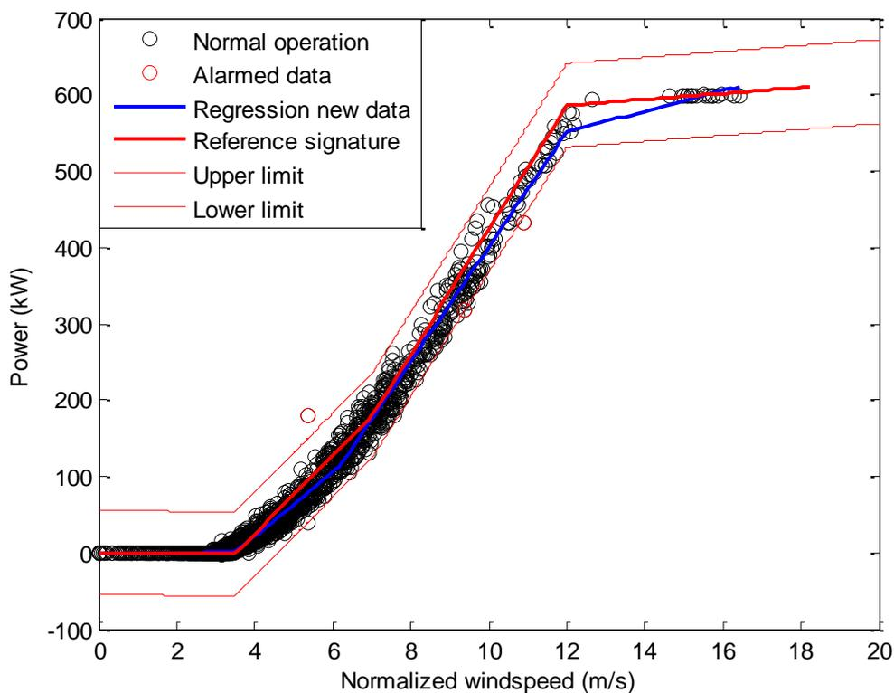
**Figure 5.8 Piecewise linear regression (4 lines) with constant limit concept for alarm generation. The data displayed is measured in the SSW direction, May 2010 - October 2010. Data points outside of the upper and lower limit would cause an alarm.**
