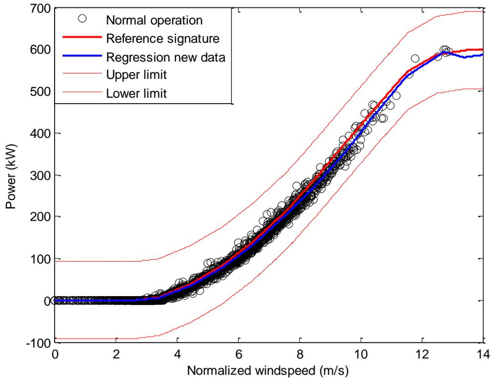
**Figure 6.1** Result of the method of bins for parameterization and constant limits concept for alarm generation, using data measured in direction S. With an alarm factor of 3, no alarm is initiated.
