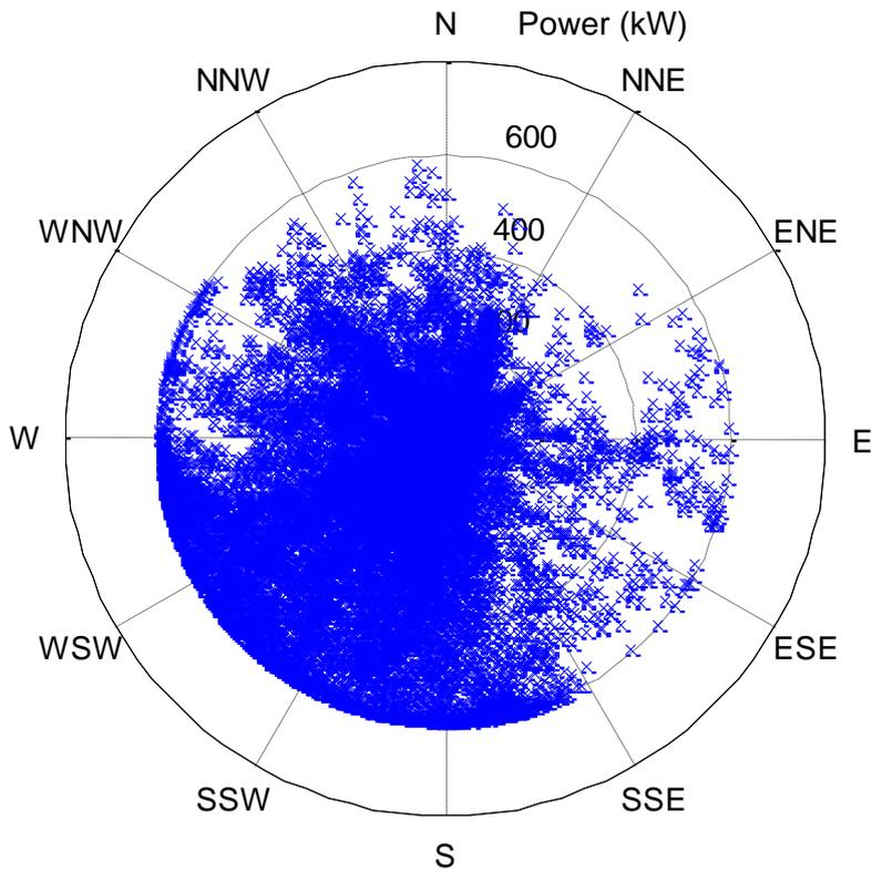
**Figure 4.4** Distribution of wind directions of measured power from Boel during June 2008 until March 2009.
