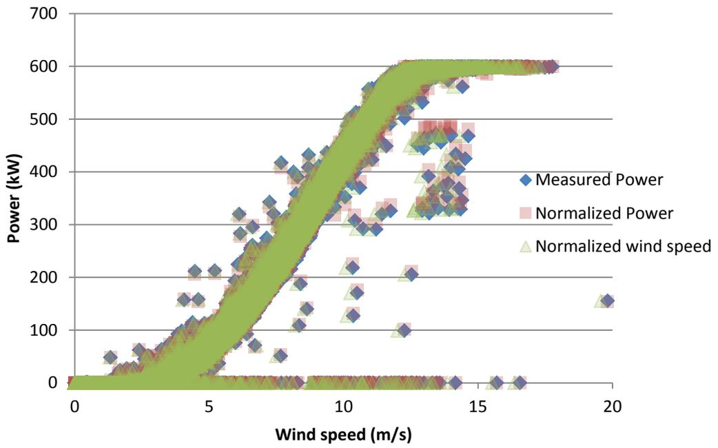
Figure 4.8 Power curves for measured power, normalized power and normalized wind speed.
