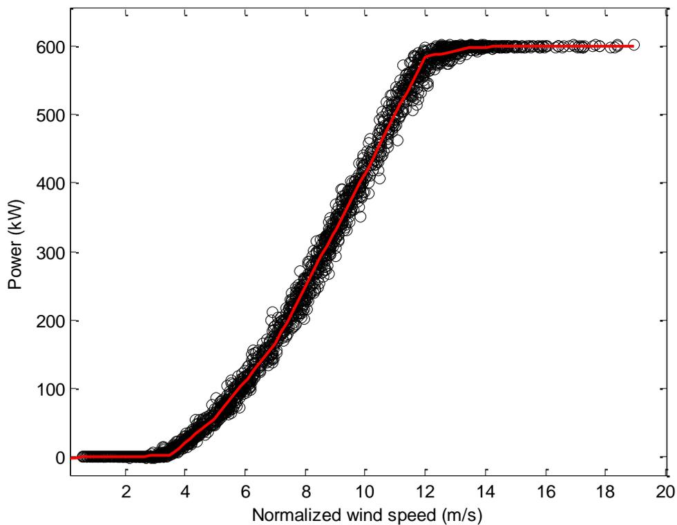
**Figure 5.3 Seven pieces, piecewise linear regression of data measured in southerly (S) winds at Boel between 2008-07-01 and 2009-03-15.**
