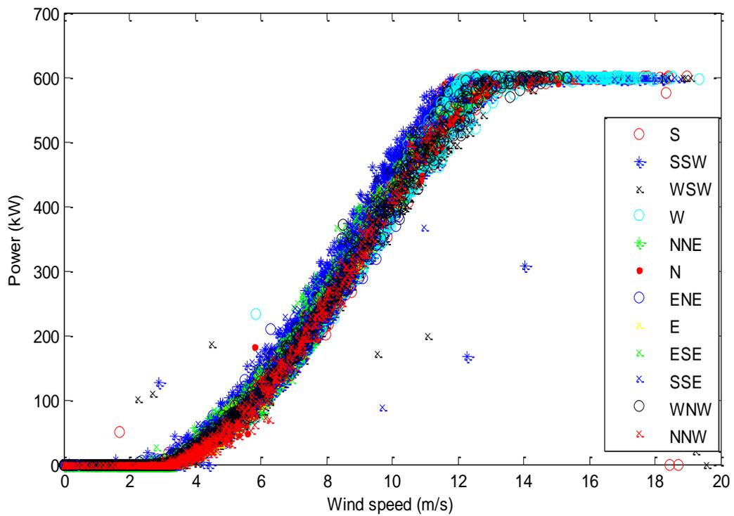
**Figure 4.5** Power output for each wind direction from the wind turbine Boel.
