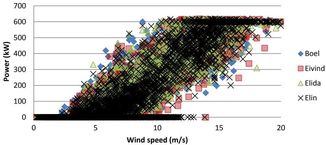
Figure 4.1 Power generated plotted against wind speed measured at the wind mast.
