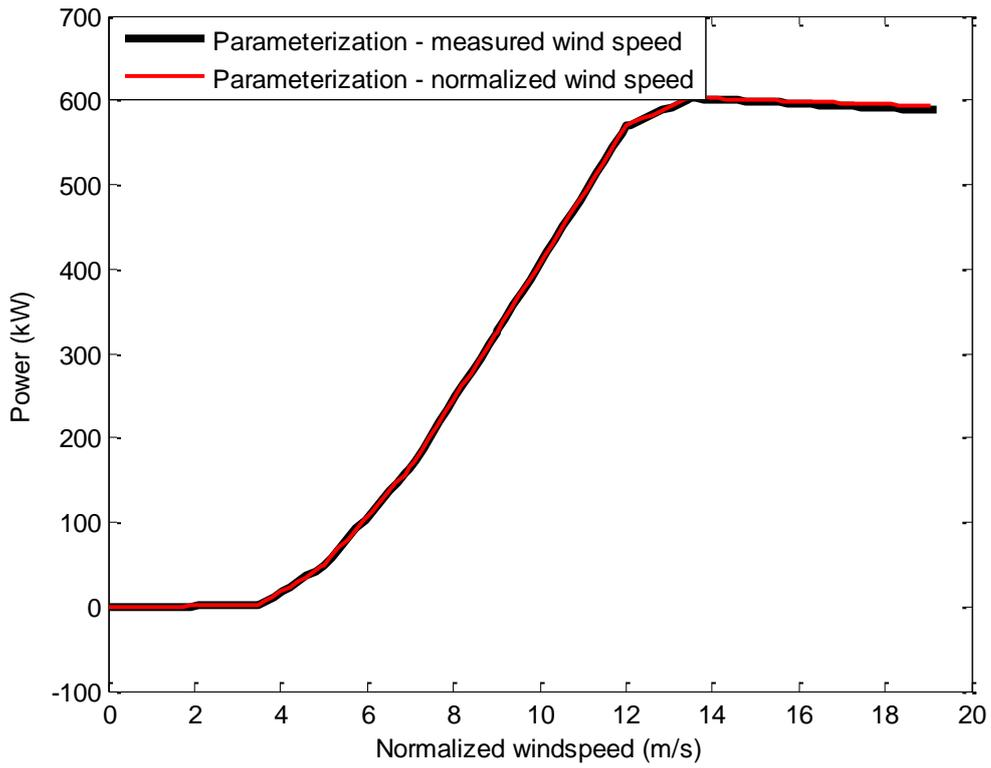
Figure 7.1 Piecewise linear regression (7 lines) of both data with normalized wind speed, and non-normalized wind speed.
