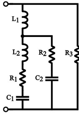
Fig. 5.6: Equivalent circuit of the plastic film capacitor ( $100nF$ ).
