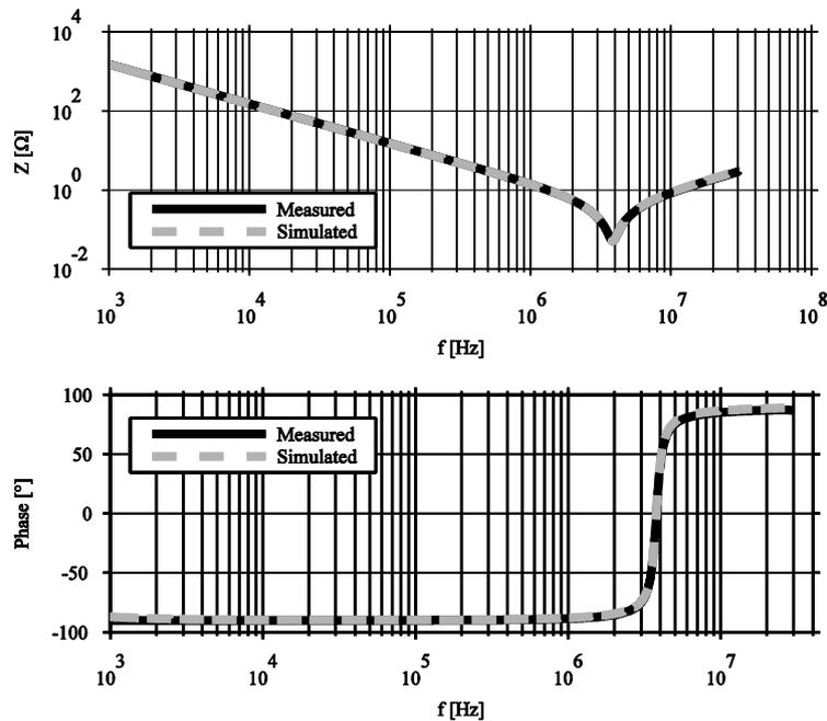
Fig. 5.5: The impedance and phase plot of the measured and modeled plastic film capacitor ( $100nF$ ).
