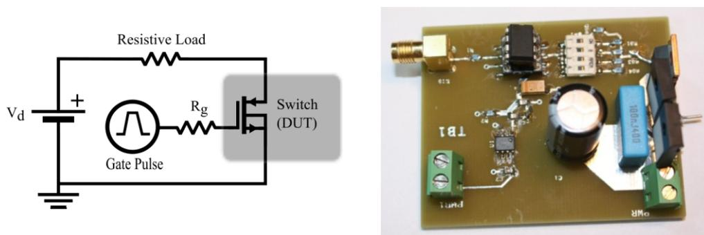
Fig. 3.2: The simplified schematic and the physical resistive load platform.
