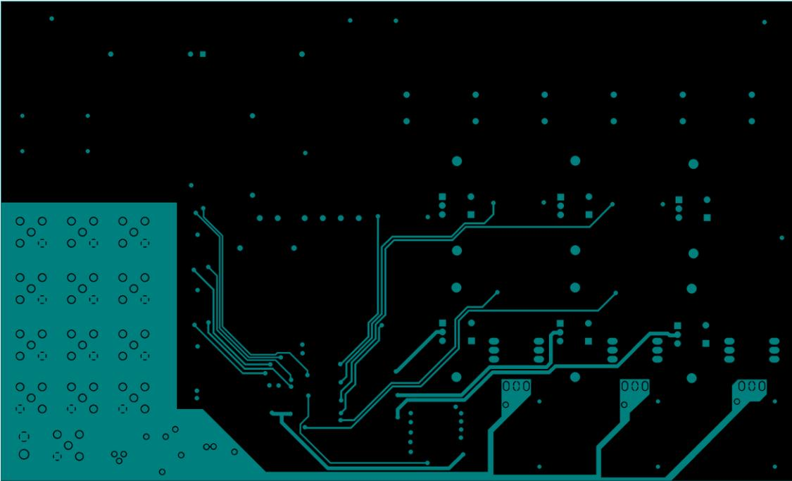
*Fig. E.4:* The third PCB layer of the three-phase inverter.
