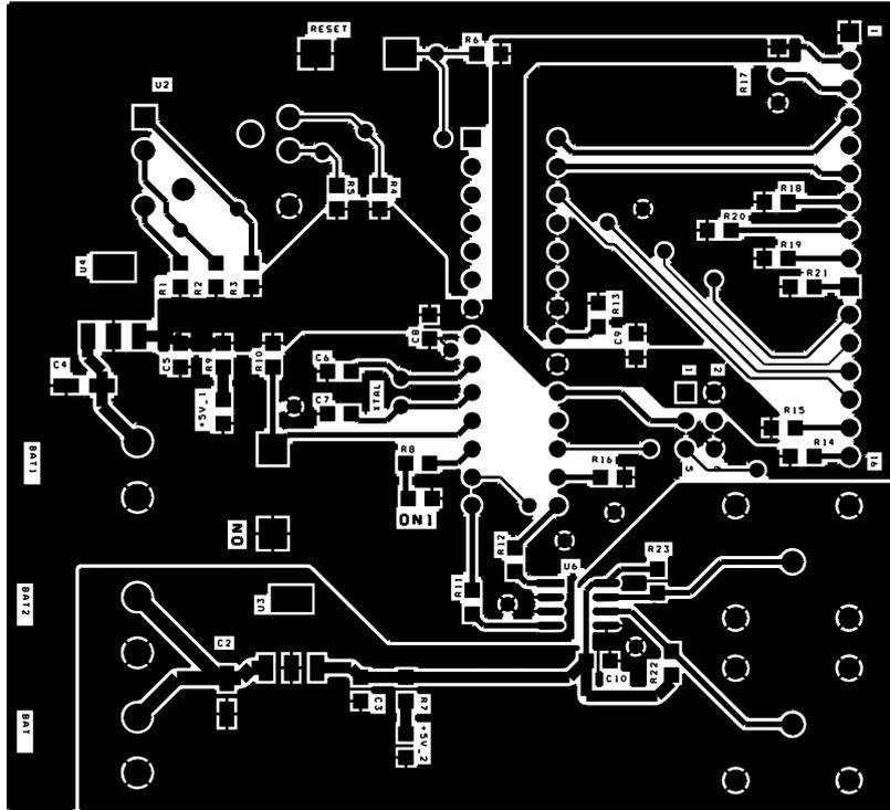
Fig. A.2: The top PCB layer of the signal pulse generator.
