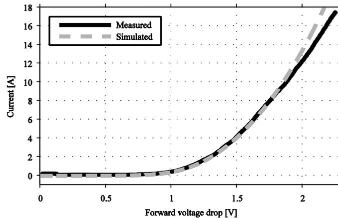
Fig. 5.11: The simulated forward current and the measured forward current.
