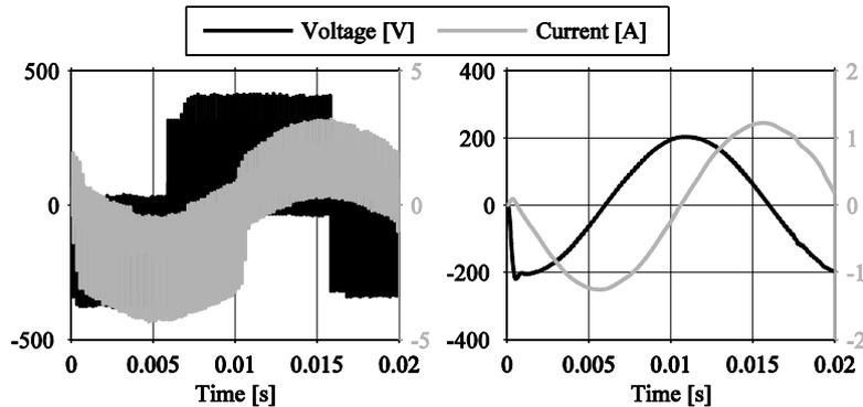
Fig. 6.6: Measured and filtered line to line voltage and phase current of loaded induction motor.
