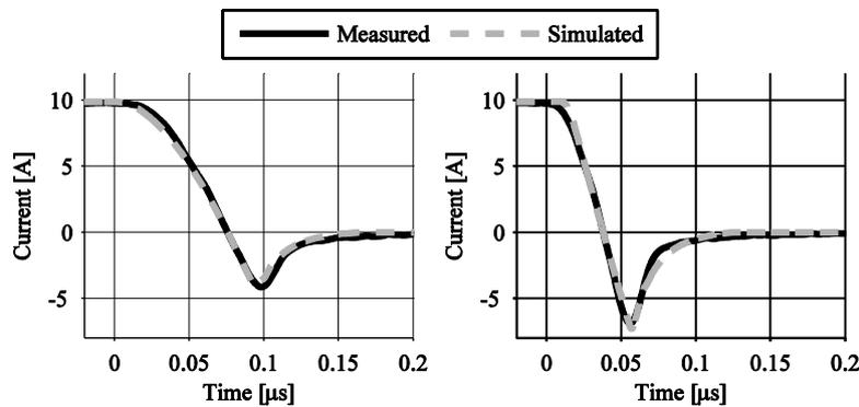
Fig. 5.15: Simulated and measured reverse recovery current. Left:  $Rg = 33\Omega$ , Right:  $Rg = 10\Omega$ .
