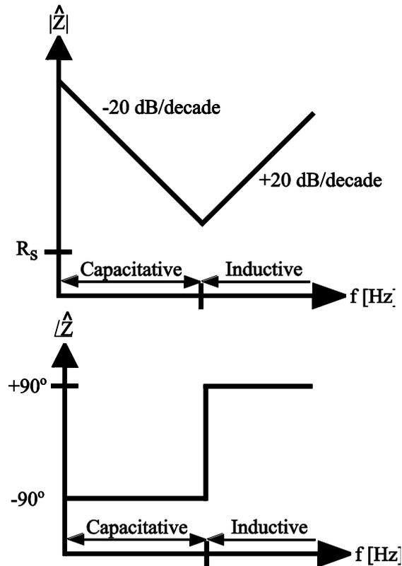
Fig. 2.4: Amplitude and phase of a non-ideal capacitor as a function of frequency.
