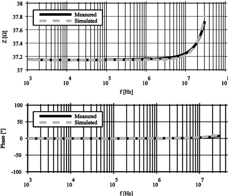
Fig. 5.1: Comparison of measured and simulated impedance and phase of the resistor ( $37\Omega$ ).
