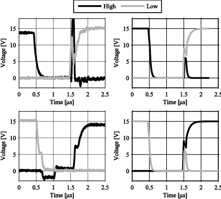
Fig. 6.9: Upper gate-emitter voltages for phase one during positive phase current. Left: measured Right: simulated
