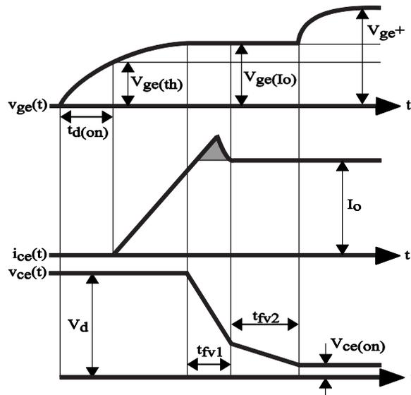
Fig. 2.10: Turn-on sequence of IGBT in test circuit with inductive load and non-ideal diode. The non ideal characteristics are shown in the shaded area.
