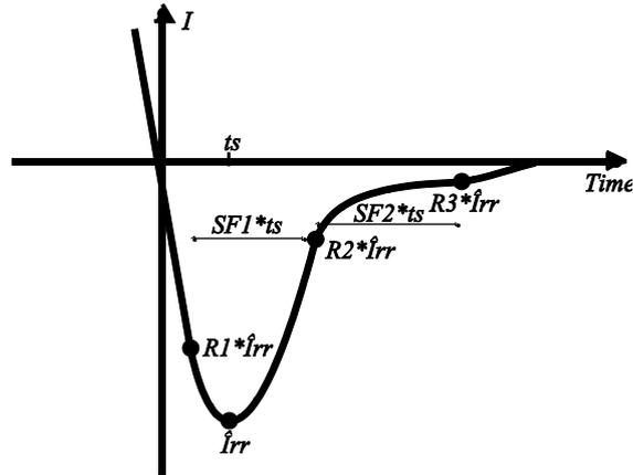
Fig. 5.14: The reverse recovery current with its different parts.
