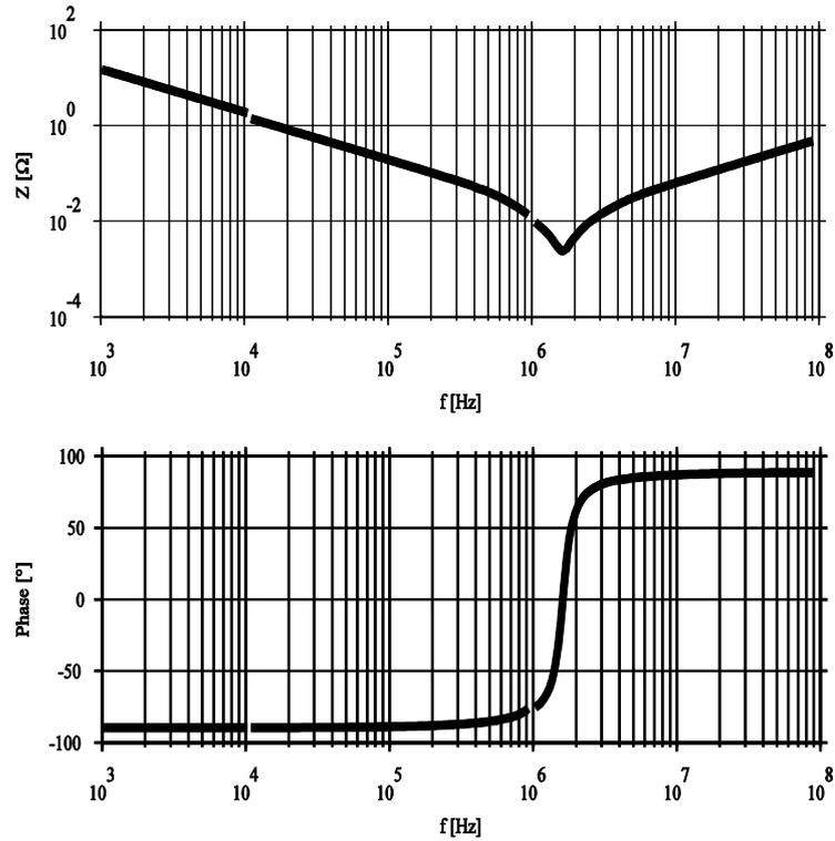
Fig.2.13: Impedance and phase response of a KEMET plastic film capacitor.
