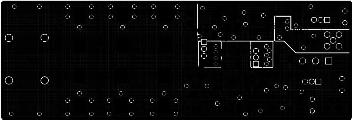
*Fig. D.3:* The bottom PCB layer of the ramp-up platform.
