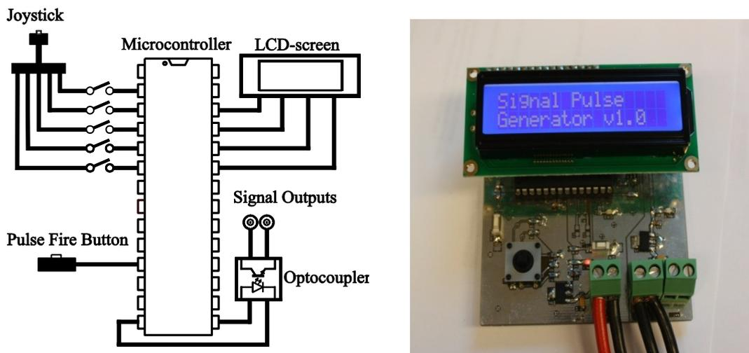
Fig. 3.1: The simplified schematic and the physical signal pulse generator.
