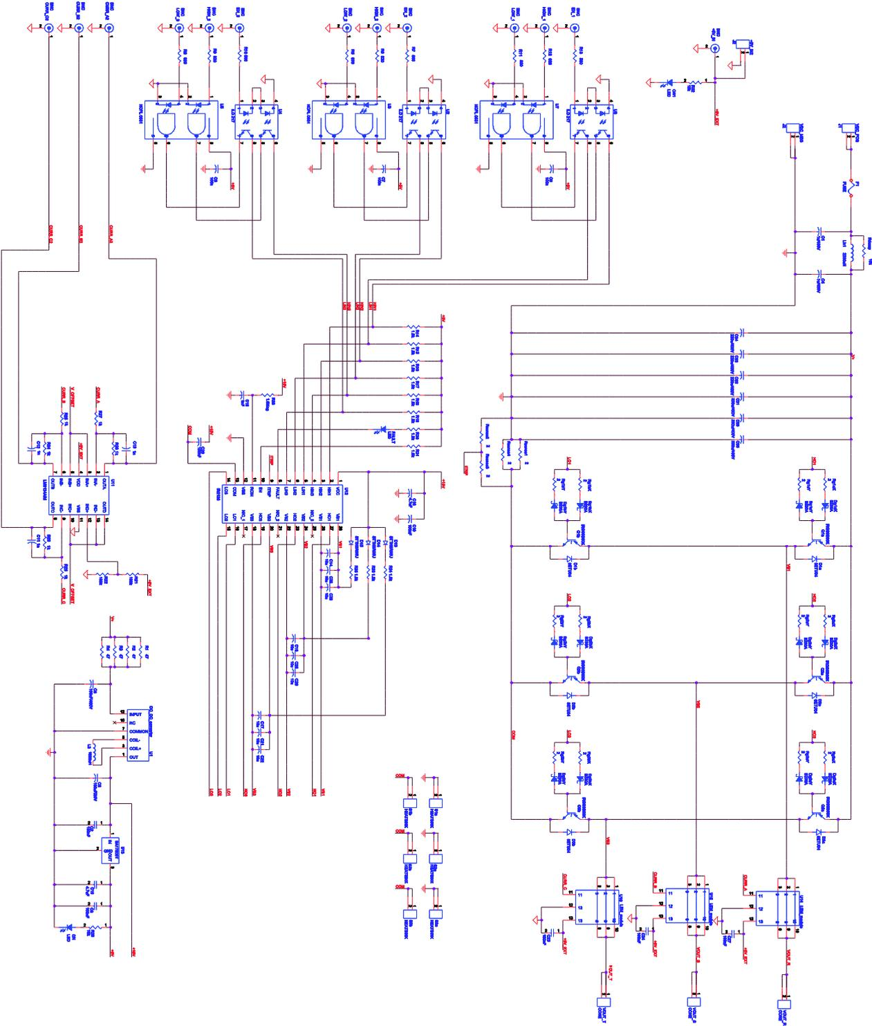
Fig. E.1: The three-phase inverter circuit schematic.
