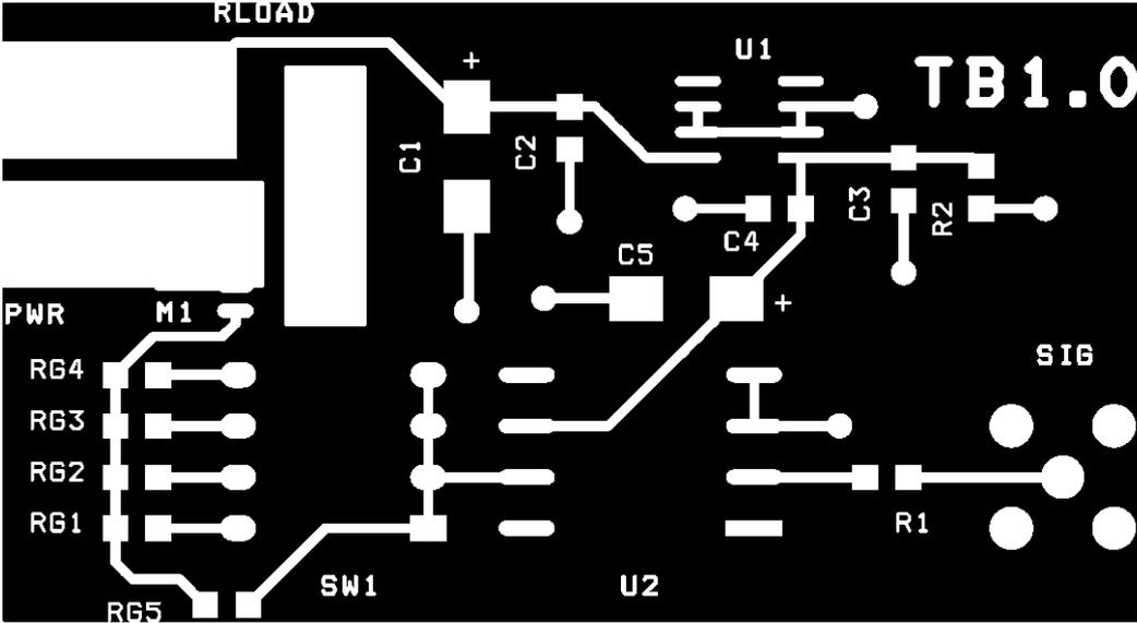
Fig. B.1: The top PCB layer of the resistive load platform.
