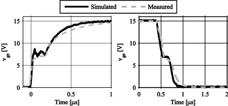
Fig.5.18: The gate-emitter voltage at turn-on and turn-off for the resistive test platform.
