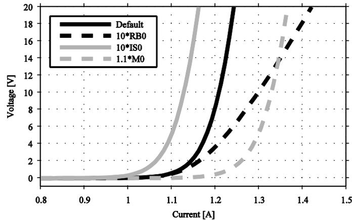
Fig. 5.10: Diode forward current with different parameters.
