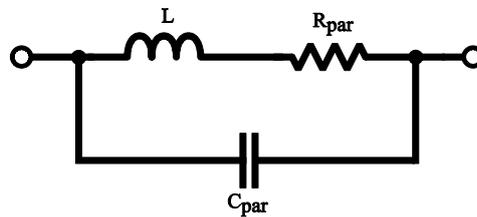
*Fig. 2.5:* Simplified equivalent circuit of an inductor using lumped parameters.
