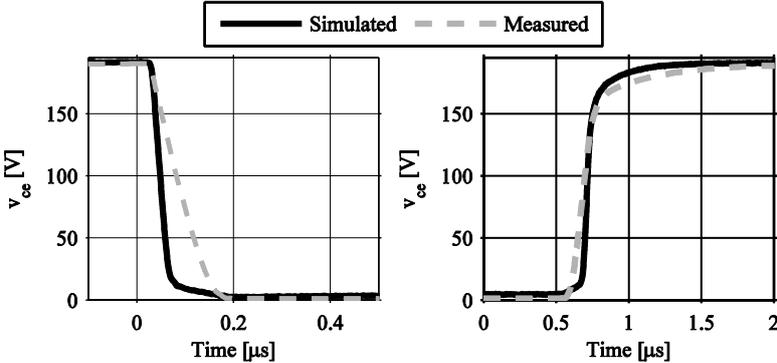
Fig.5.17: The collector-emitter voltage at turn-on and turn-off for the resistive test platform.
