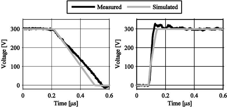
Fig. 6.7: Upper switching unit voltage during positive phase current.
