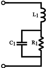
Fig. 5.2: Equivalent circuit of the resistor ( $37\Omega$ ).
