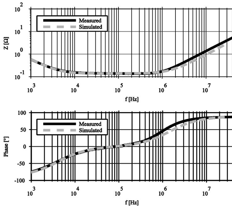
Fig. 5.7: The impedance and phase plot of the measured and modeled electrolytic capacitor ( $330\mu F$ ).
