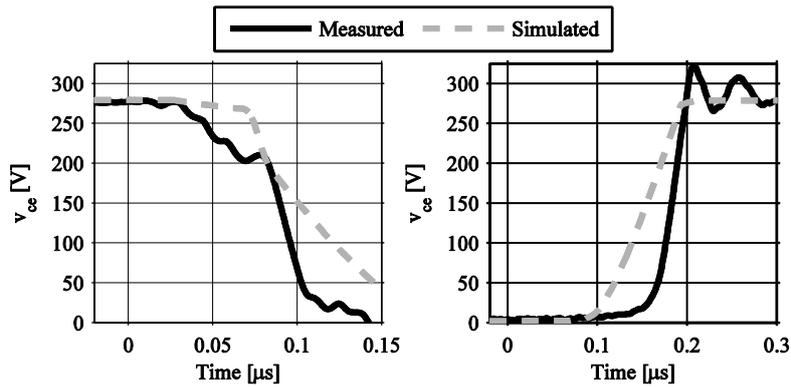
Fig. 5.20: The collector-emitter voltage for the inductive test platform at turn-on and turn-off.
