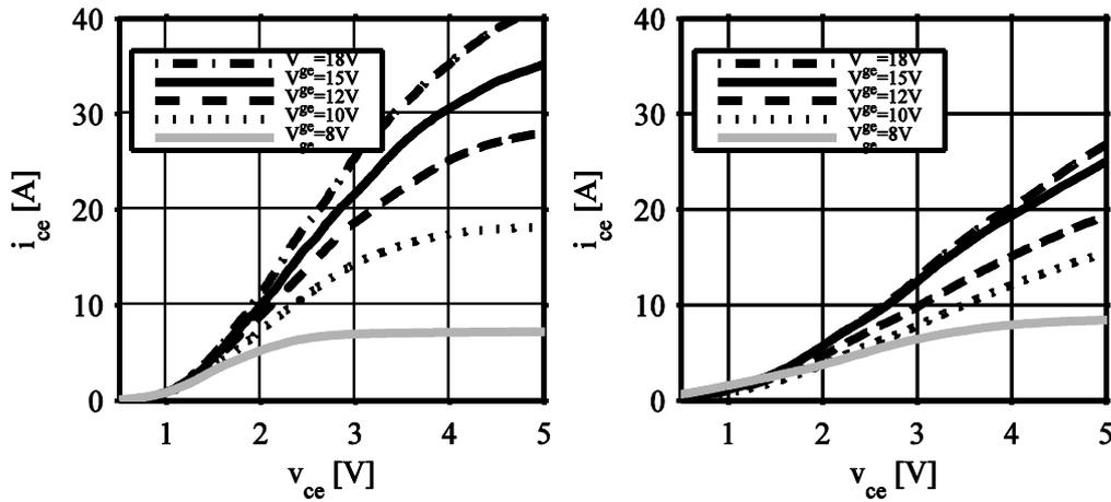
Fig. 4.7: Smoothed measured data of  $i_{ce}$  as a function of  $v_{ce}$ . Left:  $T_c = 22^\circ\text{C}$  Right:  $T_c = 150^\circ\text{C}$ .
