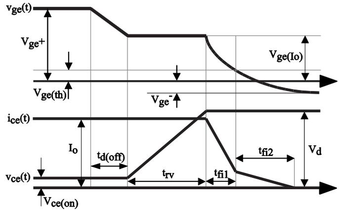
Fig.2.11: Turn-off sequence of an IGBT with the inductive load platform.
