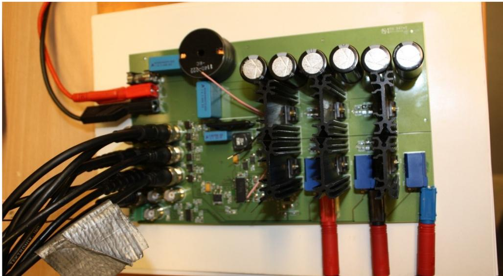
*Fig. 6.3:* The constructed three-phase inverter.
