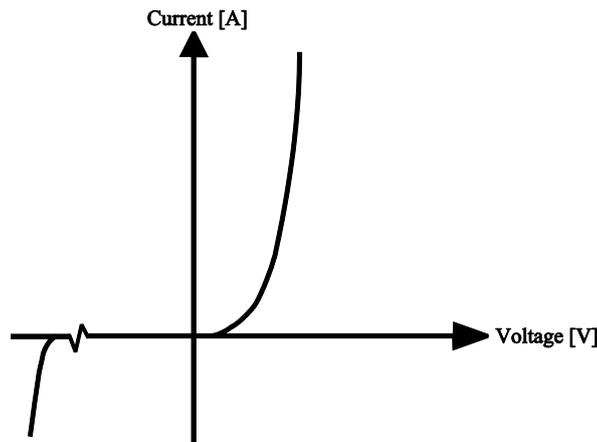
Fig. 2.7: Realistic current-voltage characteristics for different diode models.
