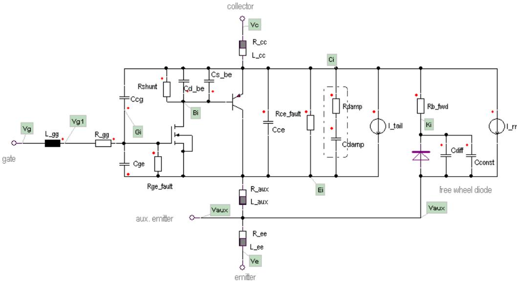
Fig.5.16: The Advanced Dynamic model in Simplorer.
