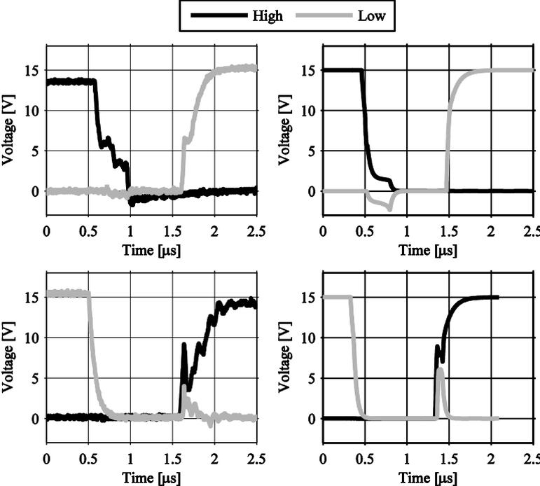
Fig. 6.10: Upper gate-emitter voltages for phase one during negative phase current. Left: measured Right: simulated
