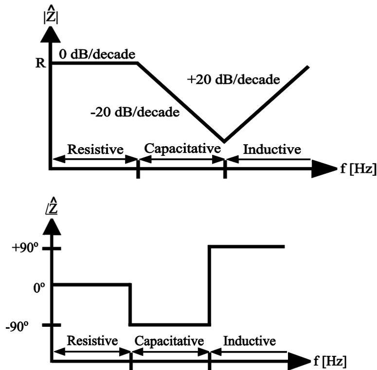
Fig. 2.2: Amplitude and phase of a non-ideal resistor as a function of frequency.
