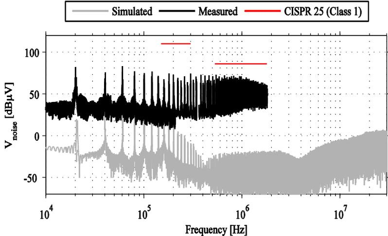
Fig. 7.2: The simulated and measured total conducted EMI.
