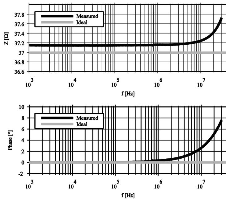
Fig. 4.1: Impedance and phase of a  $37\Omega$  resistor.
