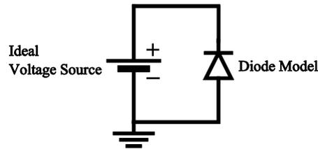
Fig. 5.12: Simple simulation setup used when determining the junction capacitance.
