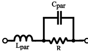
Fig. 2.1: Simplified equivalent circuit of a resistor using lumped parameters.
