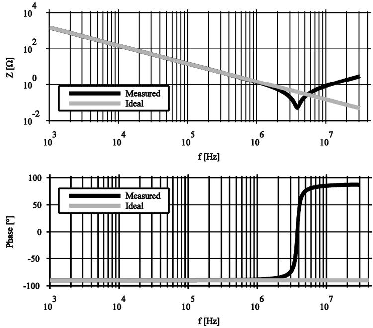
Fig. 4.3: Impedance and phase of a  $100nF$  plastic film capacitor.
