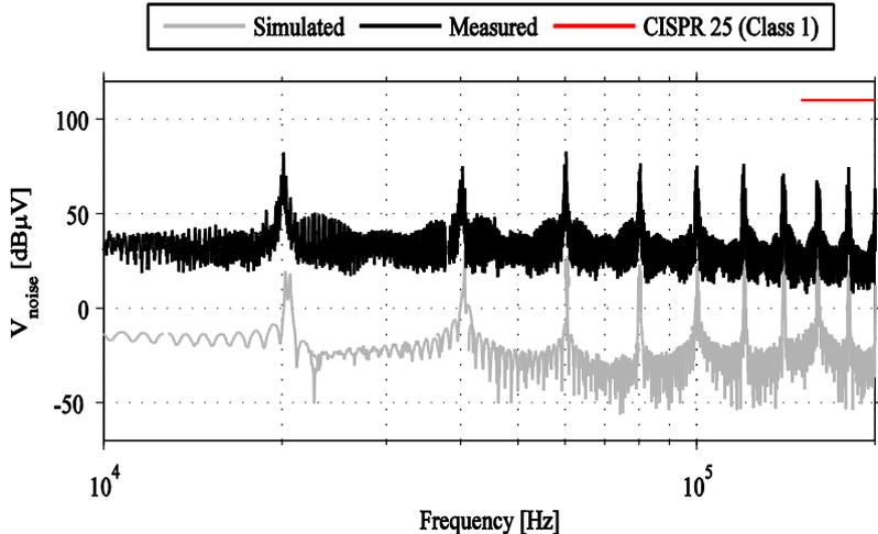
Fig. 7.3: The simulated and measured total conducted EMI in the frequency range of 10kHz to 200kHz.
