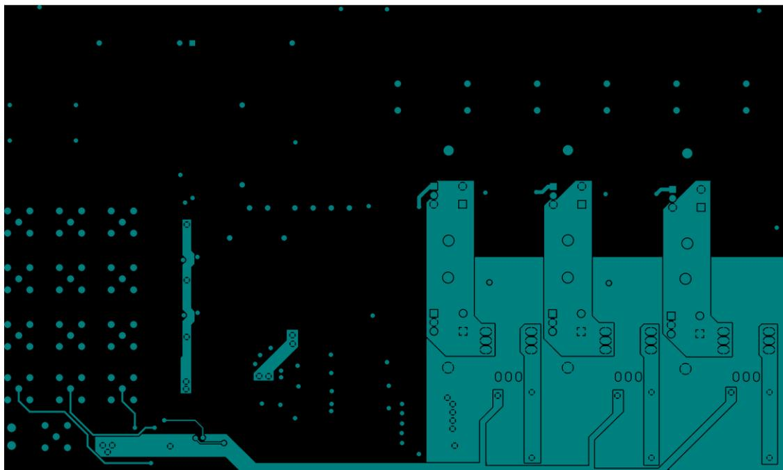
Fig. E.3: The second PCB layer of the three-phase inverter.
