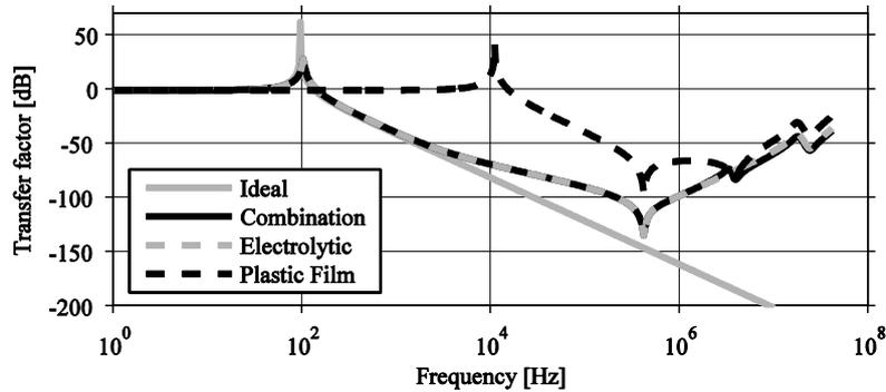
Fig. 5.9: The transfer function for different filter setups.
