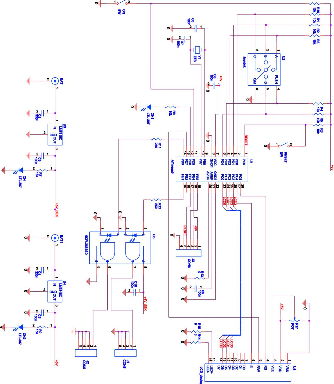
Fig. A.1: The signal pulse generator circuit schematic.
