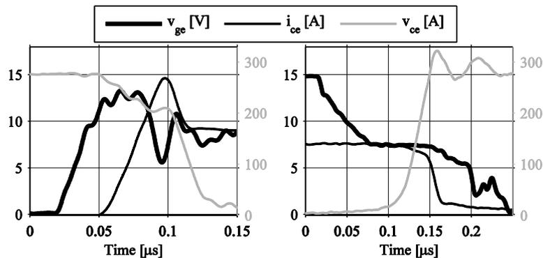
Fig. 4.9: Measured switching waveforms from the inductive load platform. Left: turn-on Right: turn-off
