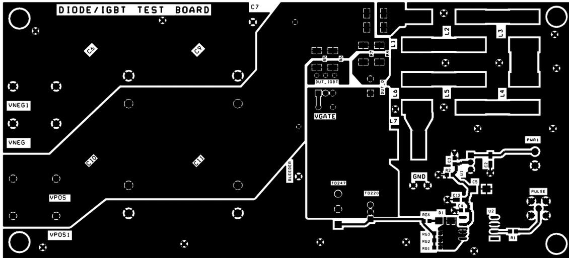
Fig. C.2: The top PCB layer of the inductive load platform.
