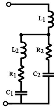
Fig. 5.8: Equivalent circuit of the electrolyte capacitor ( $330\mu F$ ).
