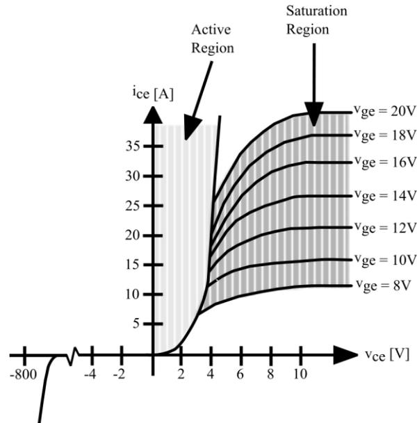
Fig. 2.9: Output characteristics of a general IGBT.
