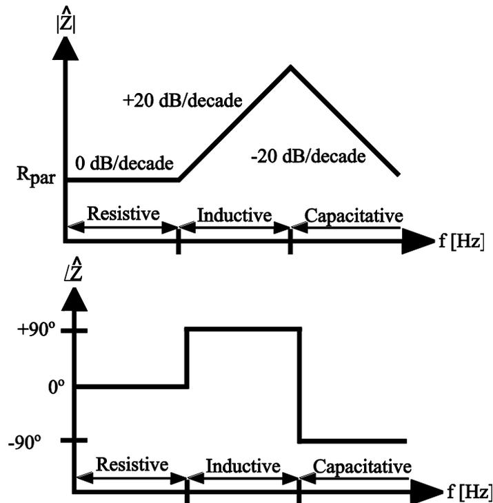
Fig. 2.6: Amplitude and phase of a non-ideal inductor as a function of frequency.
