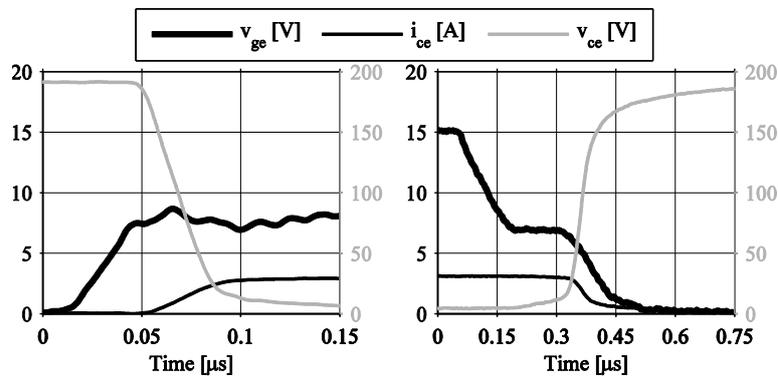
Fig. 4.8: Measured current and voltage switching waveforms from the resistive load circuit. Left: turn-on Right: turn-off
