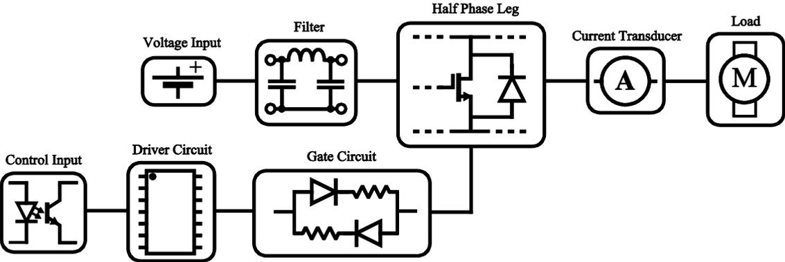
Fig. 6.2: The functional blocks of the inverter.
