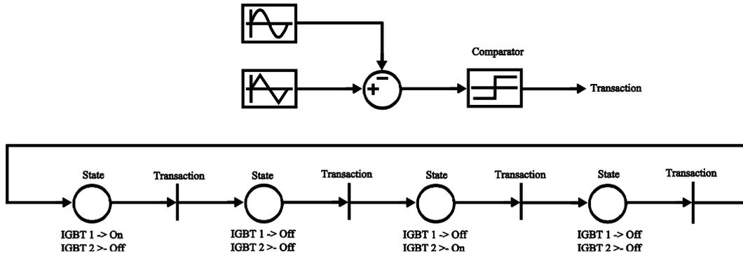
Fig. 6.5: The comparator for one phase in the inverter.
