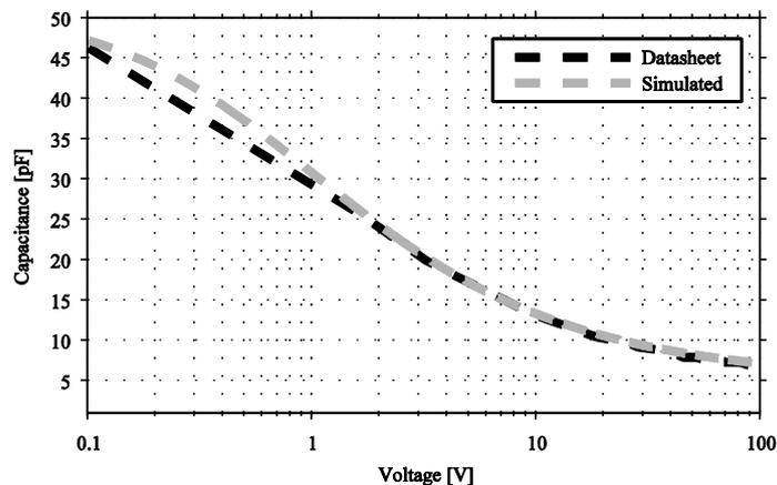
Fig. 5.13: The junction capacitance, both from datasheet and simulated.
