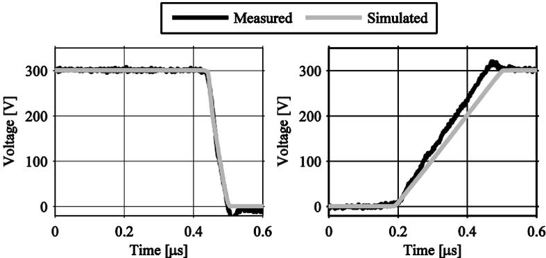
Fig. 6.8: Upper switching unit voltage during negative phase current.
