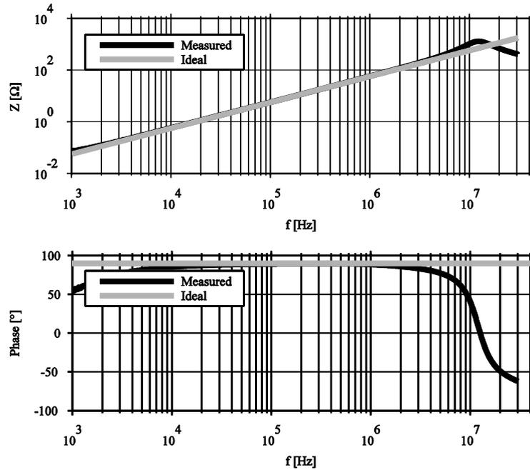
Fig. 4.2: Impedance and phase of a  $10 \mu H$  inductor.
