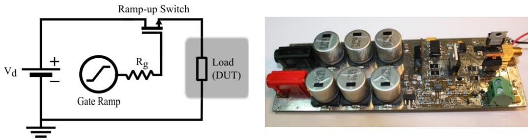
Fig. 3.4: The simplified schematic and the physical ramp-up platform.
