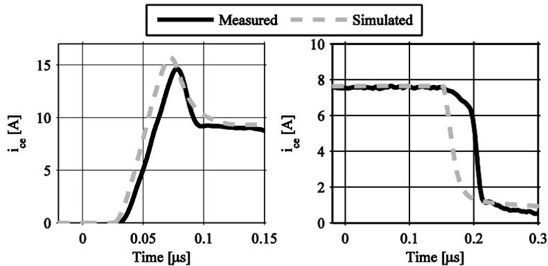
Fig. 5.22: The collector-emitter current at turn-on and turn-off for the inductive test platform.
