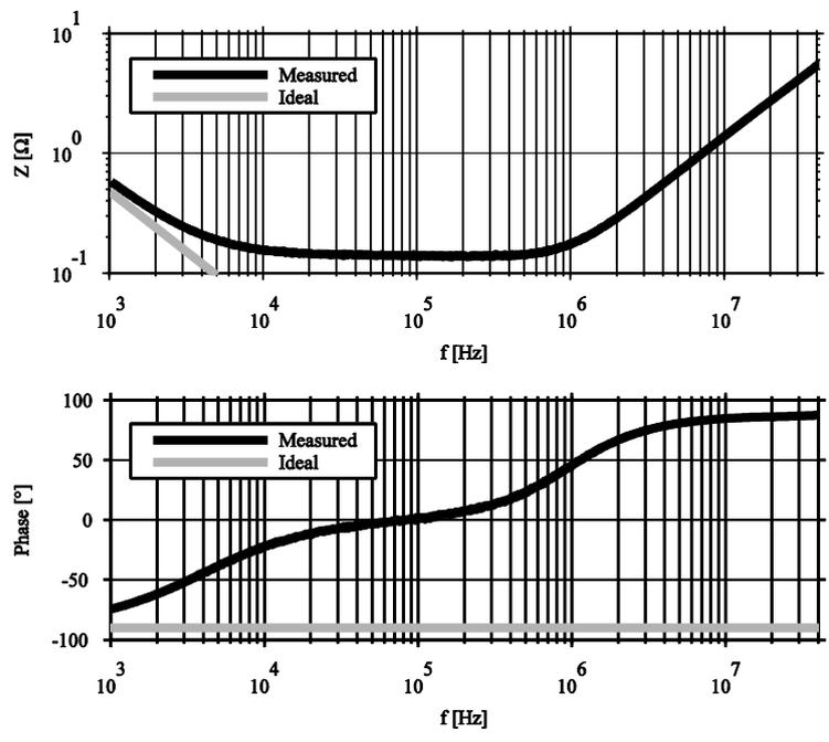
Fig. 4.4: Impedance and phase of a  $330\mu F$  electrolytic capacitor.
