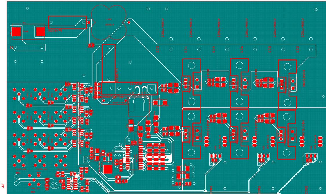
Fig. E.2: The first PCB layer of the three-phase inverter.
