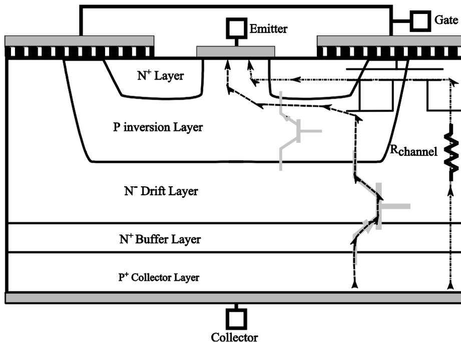
Fig. 2.8: Structure of IGBT and different conduction paths.
