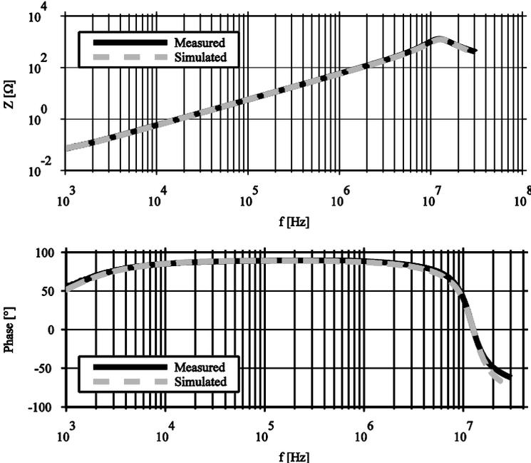
Fig. 5.3: The impedance and phase plot of the measured and modeled inductor ( $10\mu\text{H}$ ).
