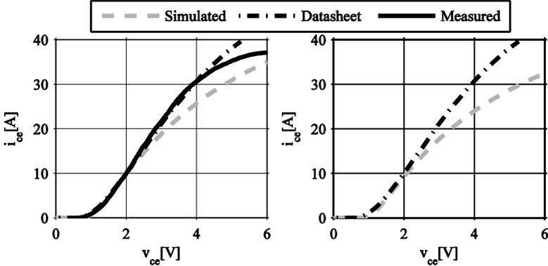
Fig. 5.23: Left:  $v_{ce}$  at  $T_c = 25^\circ\text{C}$ . Right:  $v_{ce}$  at  $T_c = 150^\circ\text{C}$ . In both cases,  $V_{ge} = 15\text{V}$
