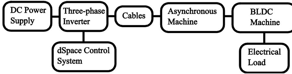
Fig. 6.4: Block diagram of the physical drive system setup.
