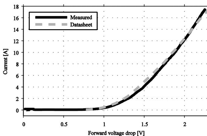
Fig. 4.5: Current/Voltage characteristics for the diode (FFPF10UP60STU).
