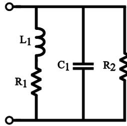
Fig. 5.4: Equivalent circuit of the inductor ( $10\mu H$ ).
