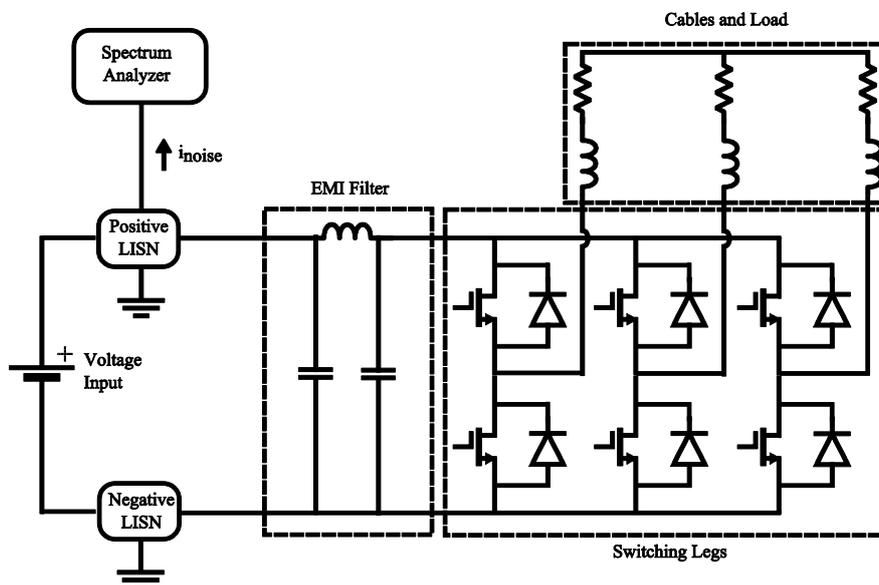
Fig. 7.1: A functional schematic of the measurement setup, including a simplified drive system.
