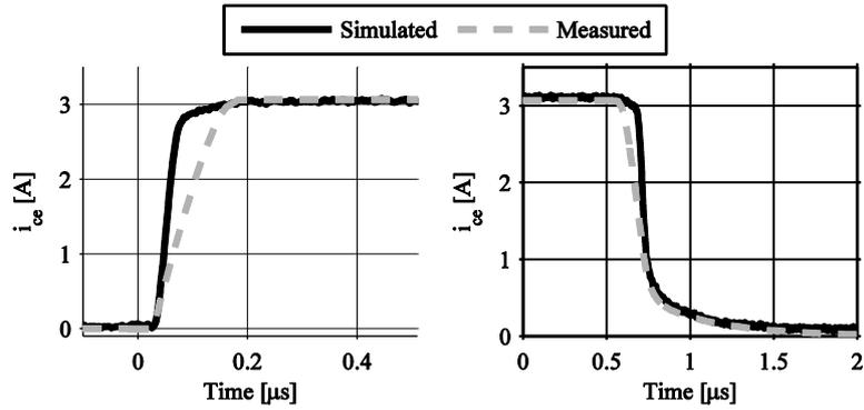
Fig.5.19: The collector-emitter current at turn-on and turn-off for the resistive test platform.
