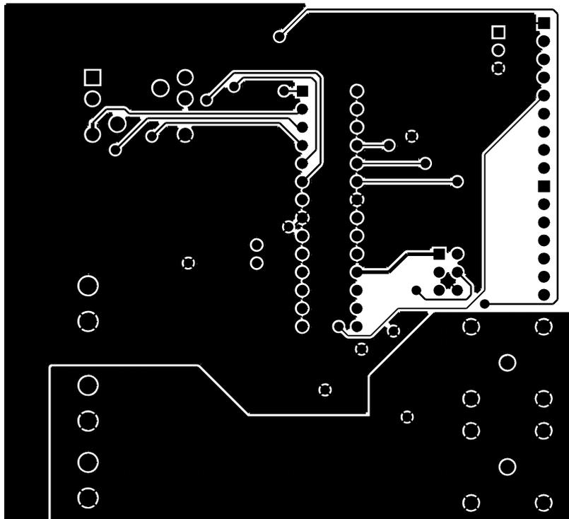
Fig. A.3: The bottom PCB layer of the signal pulse generator.
