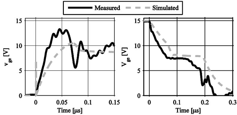
Fig. 5.21: The gate-emitter voltage for the inductive test platform during turn-on and turn-off.
