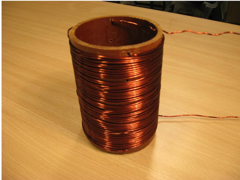
Figure 3.19: *The constructed inductor*
