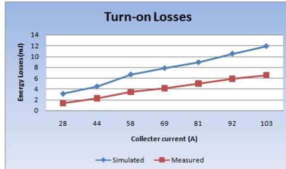
Figure 5.18: Turn-on losses for different currents
