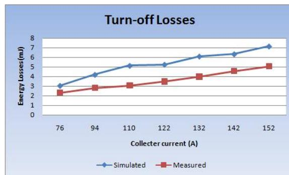
Figure 5.19: Turn-off losses for different currents
