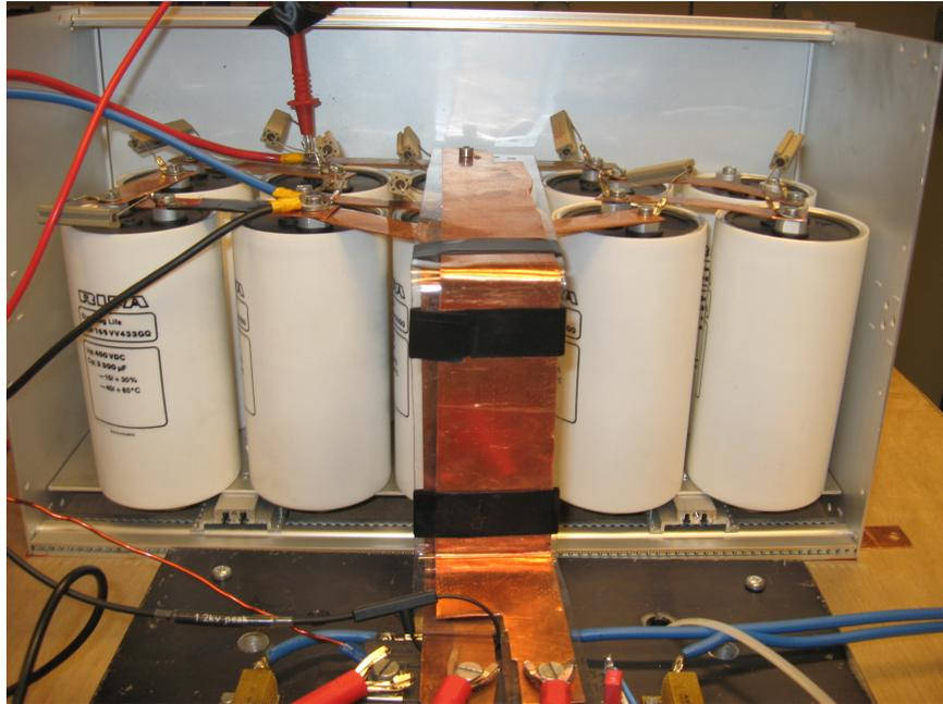
Figure 3.22: *The constructed capacitor bank*
