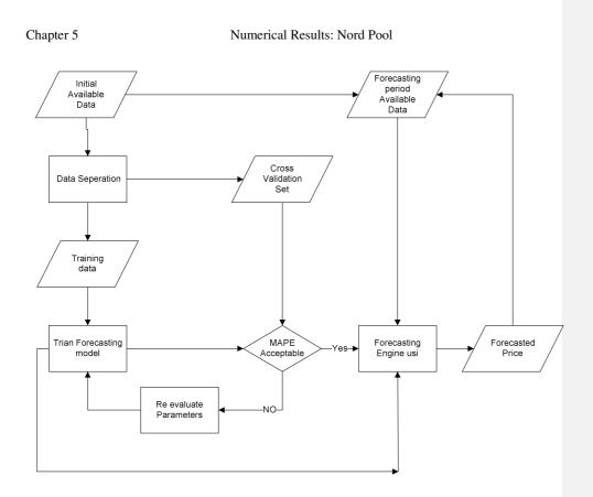
Fig. 2. Forecasting Engine Block Diagram
