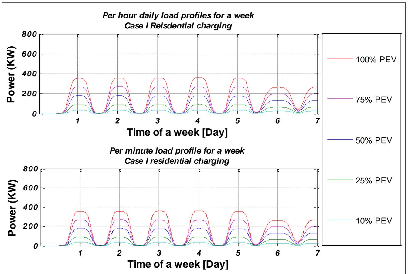
**Figure 6.45: Per hour and per minute load profiles for a week, PEV residential charging only**
