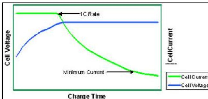
**Figure 4.5: Li-ion charging characteristics [4.3]**
