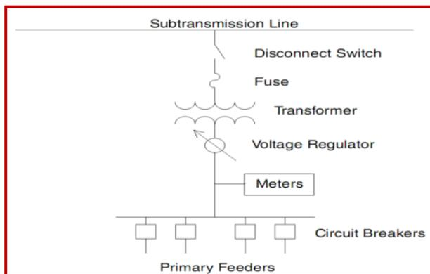
**Figure 3.3: Simple distribution substation [3.4]**
