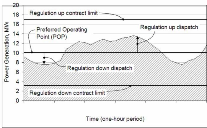
**Figure 2.1: Example power profile for a power generator providing regulation up and regulation down. The shaded area represents the energy generated over the one-hour period [2.3]**
