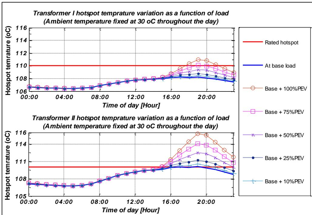
**Figure 6.53: Distribution transformer hotspot temperature profiles resulting from Case II residential charging**
