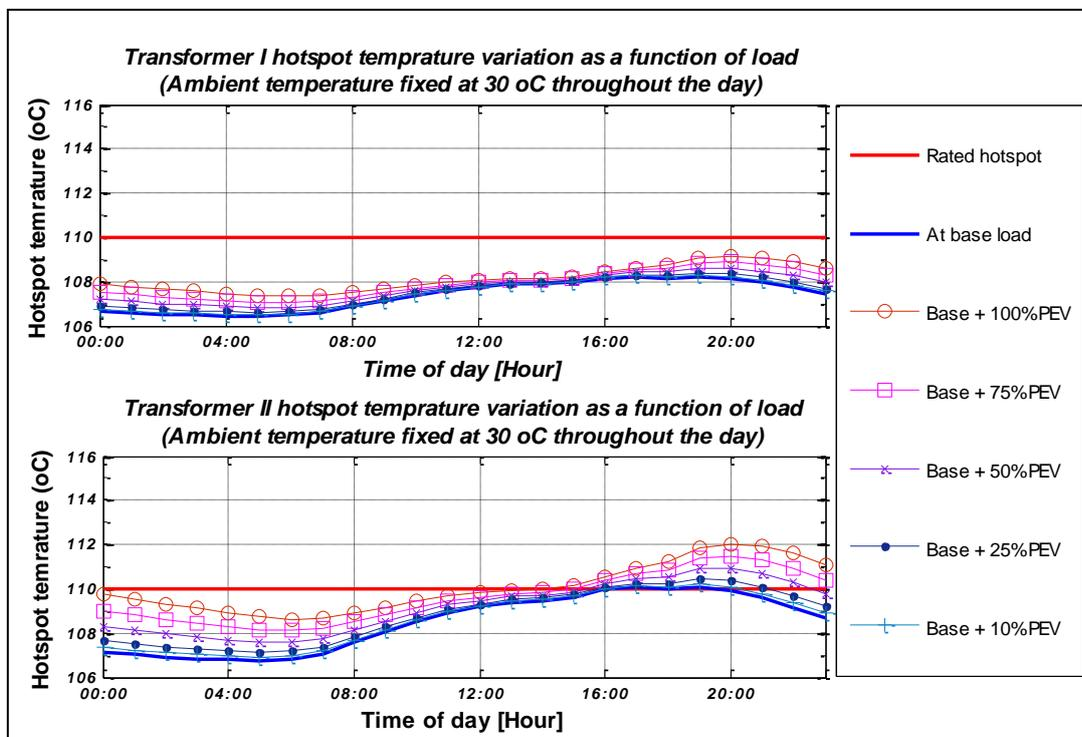
**Figure 6.48: Hot spot temperature profiles of transformers resulting from different loading condition of transformers**
