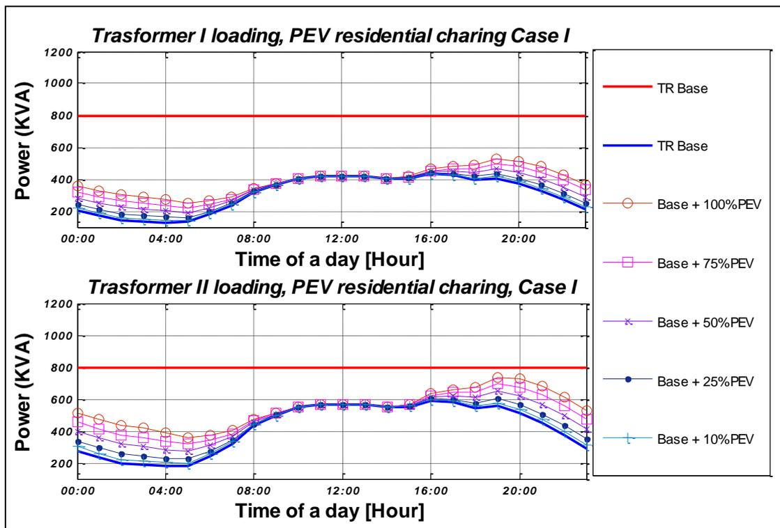
**Figure 6.47: Transformer loadings resulting from PEV residential charging**
