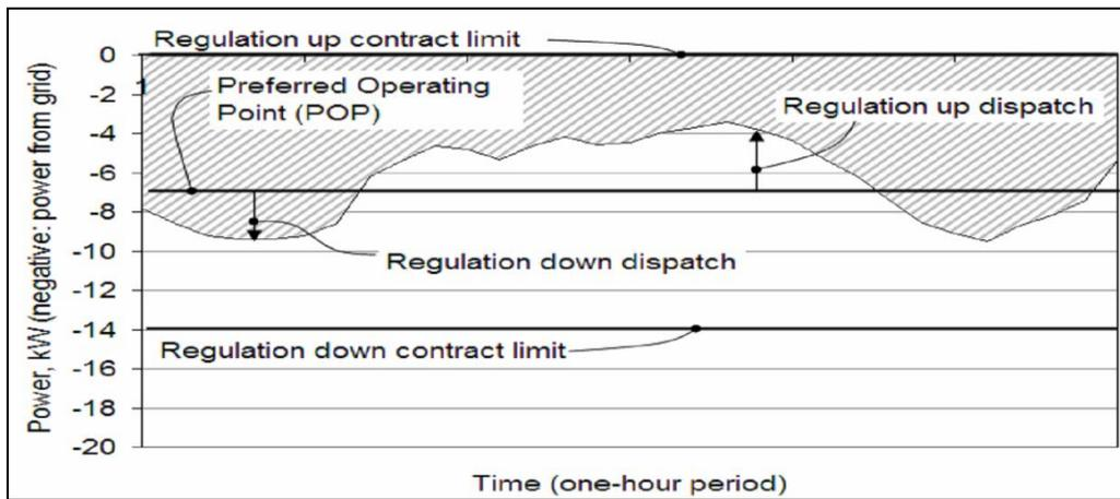
**Figure 2.3: Example power profiles for a PEVs with unidirectional chargers providing regulation up and down ancillary service with a POP value of -7kW (ie. 7 kW of load). The shaded area represents the energy delivered to the vehicle by the grid over the one-hour period [2.3]**
