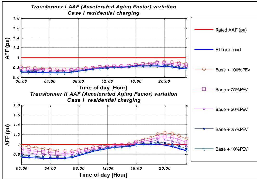
**Figure 6.49: Transformers Accelerated Aging Factors**
