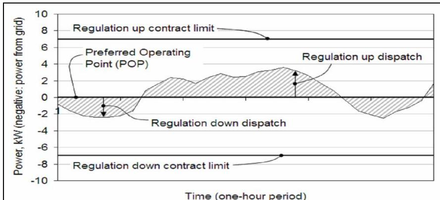
**Figure 2.2: Example power profiles for PEVs with a bi-directional charger providing regulation up and down ancillary service with a zero POP. The shaded area above zero represents energy delivered to the grid from the vehicle (regulation up) and the shaded area below zero represents the energy consumed by the vehicle (regulation down) [2.3]**
