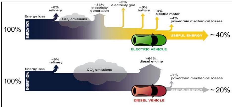
**Figure 1.7: Well-to-wheel efficiency of Electric vehicle vs. Diesel vehicle [1.11]**
