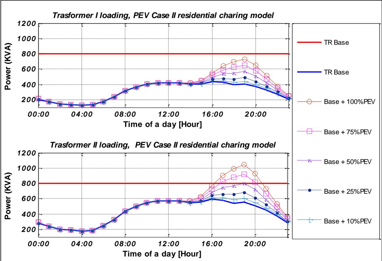
**Figure 6.52: Transformer loadings resulting from Case II residential charging**
