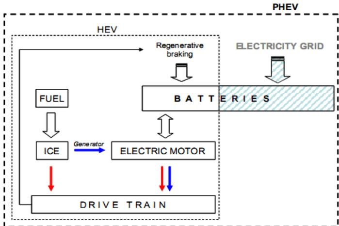
**Figure 3.7: Simplified representation of HEV/PHEV configuration (blue: series; red: parallel) [3.7]**
