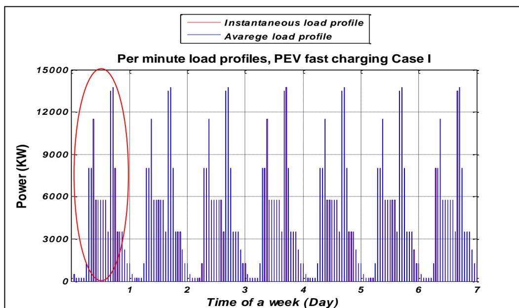
**Figure 6.3: Per minute load profile for a week, PEV fast charging at 250KW**
