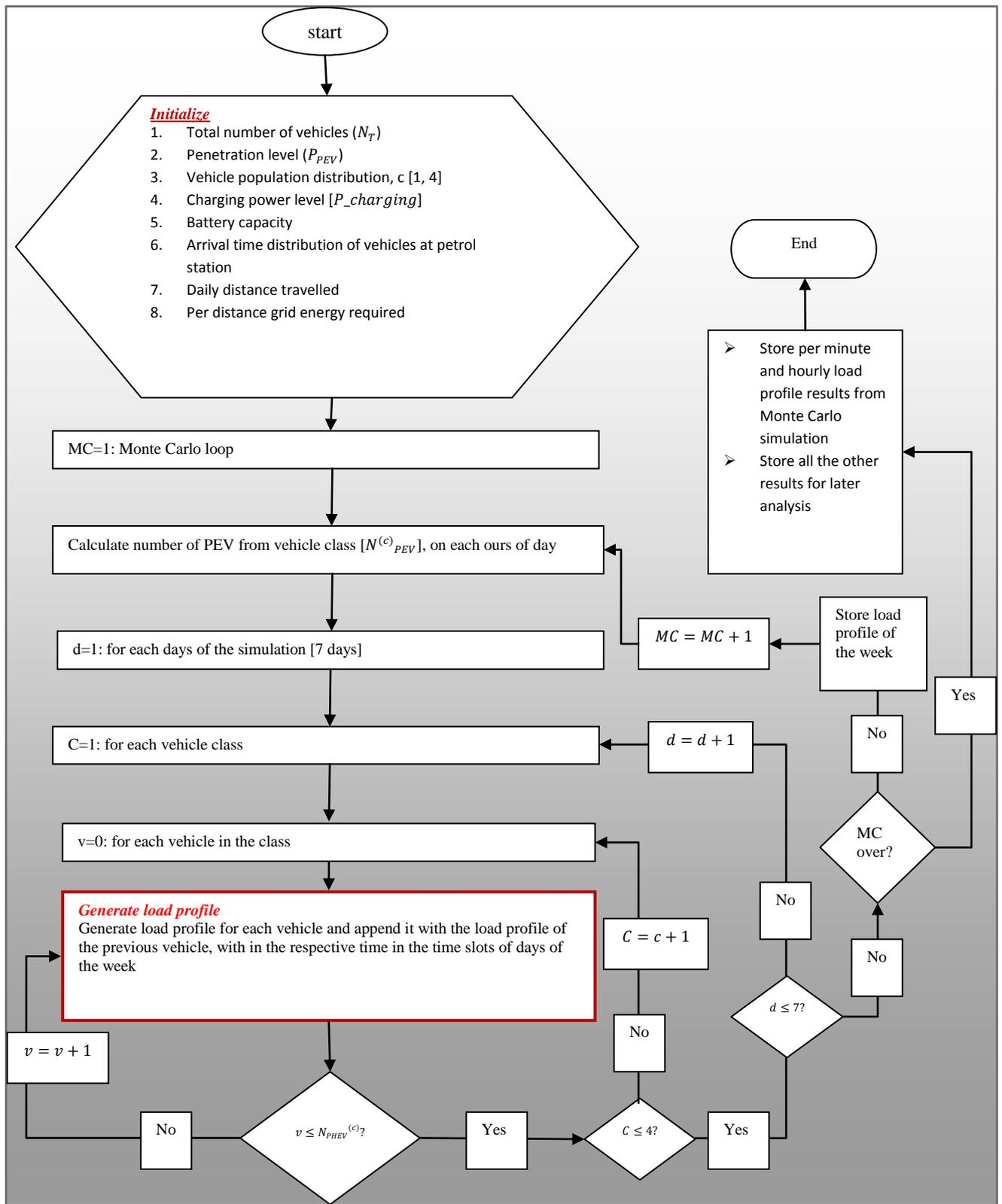
Figure 5.10: Fast charging model flow chart
