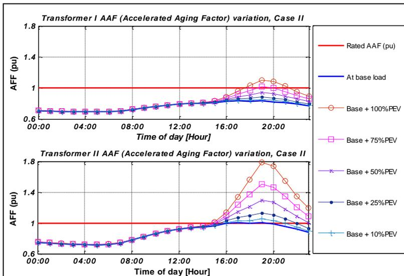
**Figure 6.54: Accelerated Aging Factors of transformers resulting from Case II residential fast charging**
