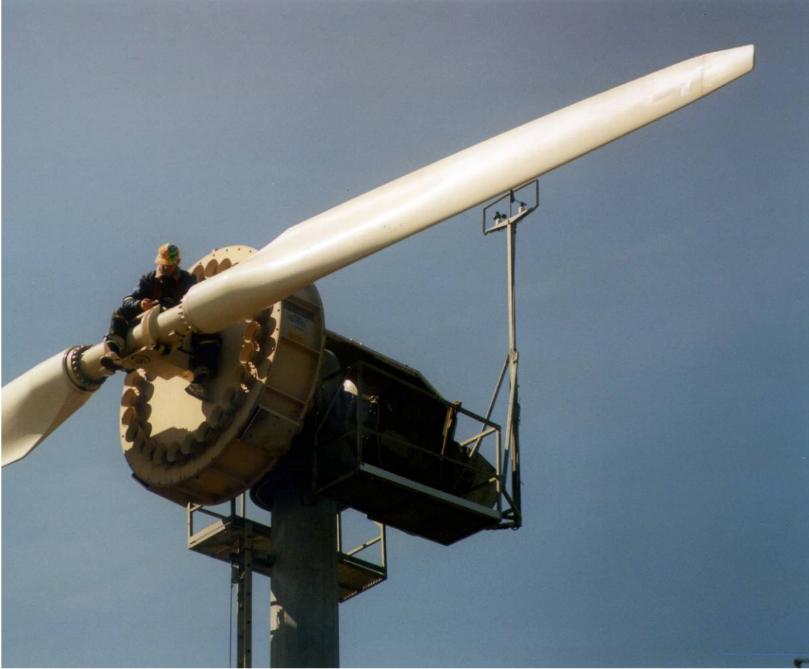
Fig. 1: Photo of the nacelle. Hub arrangement with teeter hinge is visible. The rotor is attached directly to the generator shaft. The ring of holes around the generator surface is the support tubes for the stator modules. They also serve as channels for cooling air through the generator. On the mast at the rear end of the nacelle there is an anemometer and wind vane connected to the control system.
