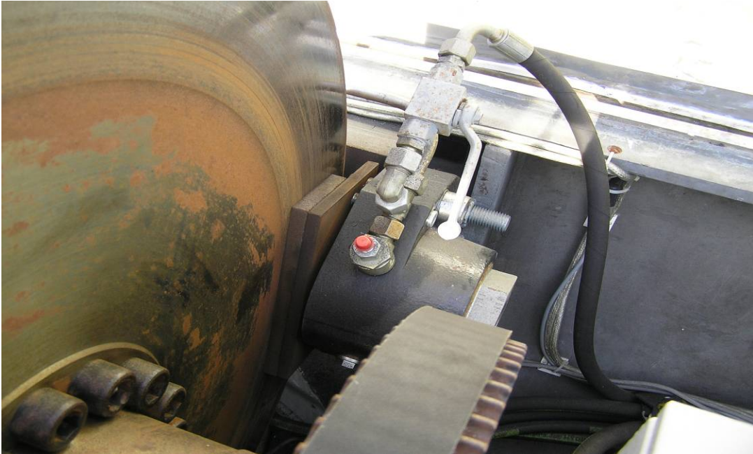
Fig. 3: Disc brake with one of the two calipers. Part of starter motor belt drive is also visible.
