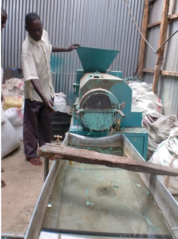
Plate 15. Picture showing a pelletizer used at the recycling plant.
