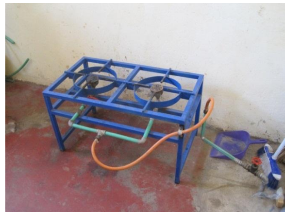
Plate 18. Picture showing a two plate burner that uses methane from the bio center
