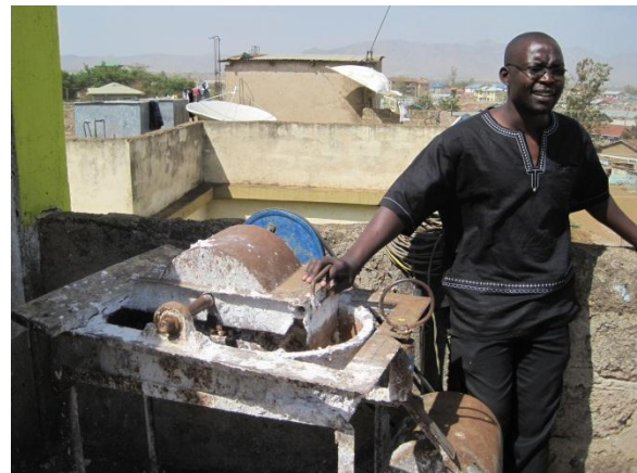
Plate 31. Picture showing the machine used to prepare the recycled paper made out of waste paper mache and the water hyacinth
