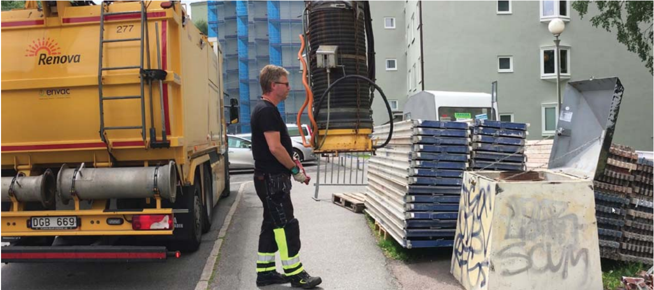
Figure 16: Waste collection of the buildings in the city centre that had the vacuum system, studied in case C. In this case the air suction is generated by the collector truck.
