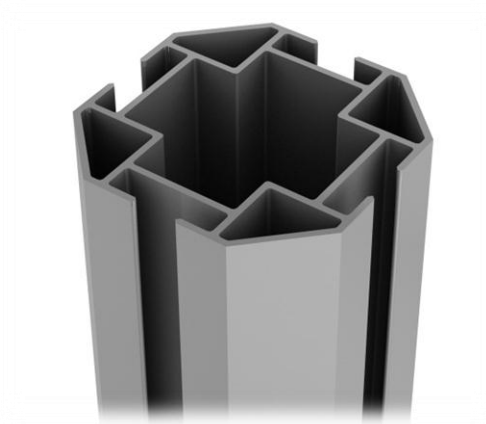
Figure 43. Part of CAD model that illustrates the pole with its four 'T'-grooves.
