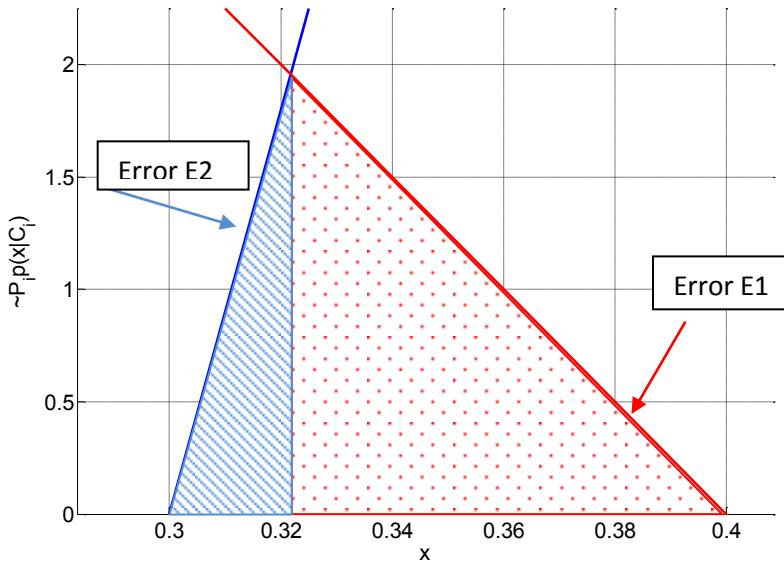
$$\text{error } E1 = 2 \int_{T_1}^{0.4} P_1 p(x|C_1) dx \quad \text{area } A1 = 2 \int_0^1 P_1 p(x|C_1) dx$$
