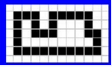
This is the boundary extracted by taking the set difference of A and its erosion
