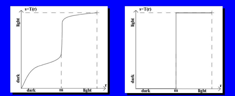
HISTOGRAM EQUALIZATION Let the variable r represent the gray level. For any r in the interval [0,1] (with r=0 representing black, and r=1 representing white), consider the transformation:
